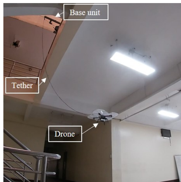
Fig. 17. Actual image of tethered drone during laboratory-based experiment.
