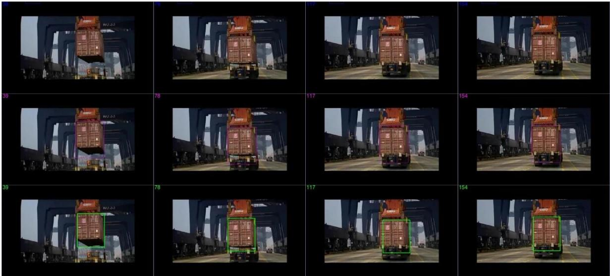
Fig. 19. Video 5 – container tracking with optimized CSK, DFT and LOT (from the top), frames 39, 78, 117, 154 taken from [36].
