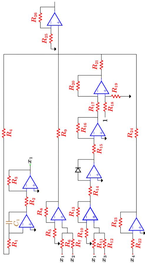
Fig. 9. Op-Amp circuit diagram of chaotic variable  $x_1$
