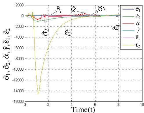
Fig. 4. The parameter estimation of the modified Colpitts oscillator
