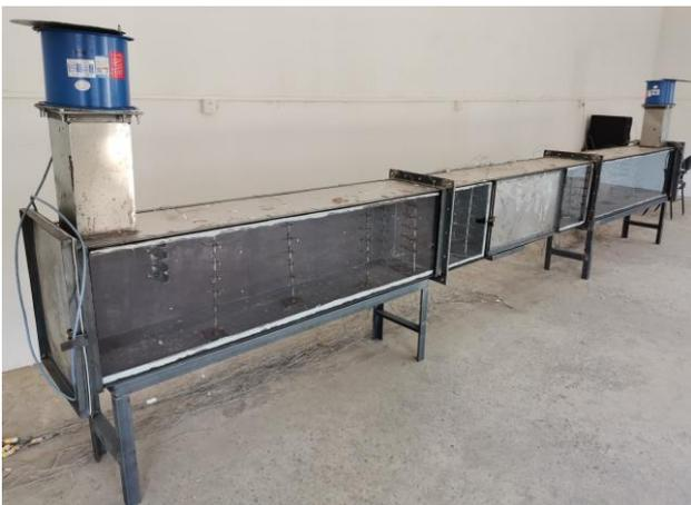
Figure 1. Physical model of cable compartment in utility tunnel
