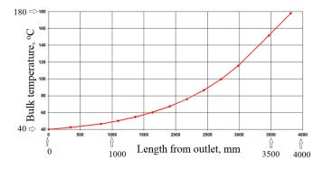
Fig. 4. Temperature gradient shell side
