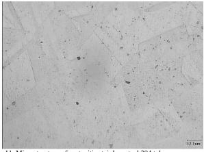
Fig. 11. Microstructure of austenitic stainless steel 304 tube
