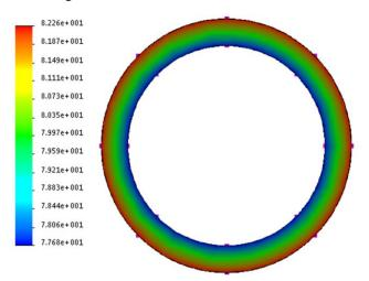
Fig. 6. Temperature distribution inside tube wall
