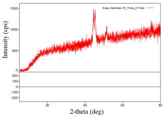
Fig. 10. X-ray diffraction result for tubes material
