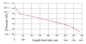
Fig. 8. Pressure Gradient tube side
