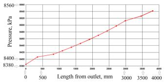
Fig. 7. Pressure Gradient shell side
