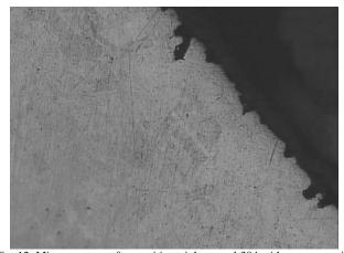
Fig. 12. Microstructure of austenitic stainless steel 304 with some porosity on the surface.
