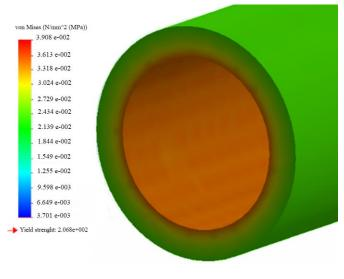
Fig. 9. Stress analysis tube side
