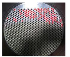
Fig. 2. Deposits of material-clogged SS 304 tubes on the top side
