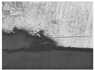
Fig. 14. Cracks start from corrosion pits.
