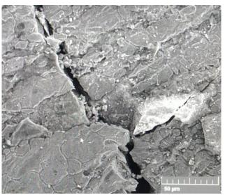
Fig. 15. SEM micrographs of Chloride stress corrosion cracking.
