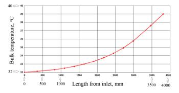
Fig. 5. Temperature gradient tube side
