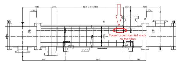
Fig. 1. Circumferential crack position in heat exchanger system.
