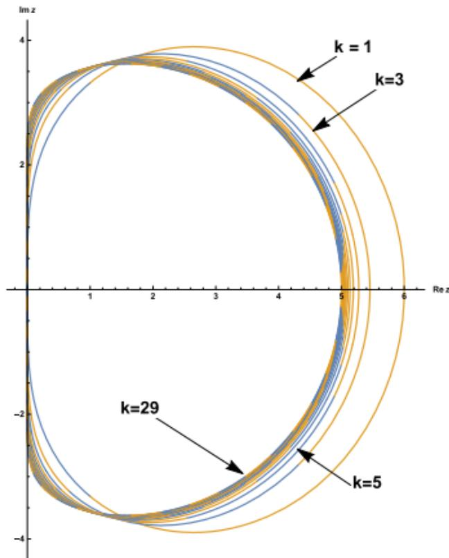
Figure 2: Stability region (exterior of closed curve) of GSDLMME in [28],  $k = 1(2)29$ . The curves are for  $k = 1, 3, 5, 7, \dots, 29$ . However, the curves for  $k = 7, 9, 11, \dots, 29$  are so close to one another that they are indistinguishable.
