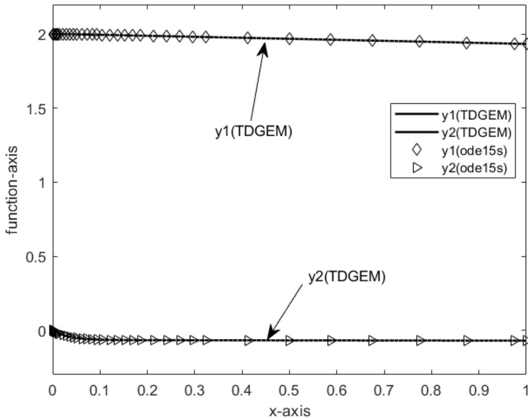
Figure 13: Numerical results for Van der Pol equation using the eighth order TDGEM.
