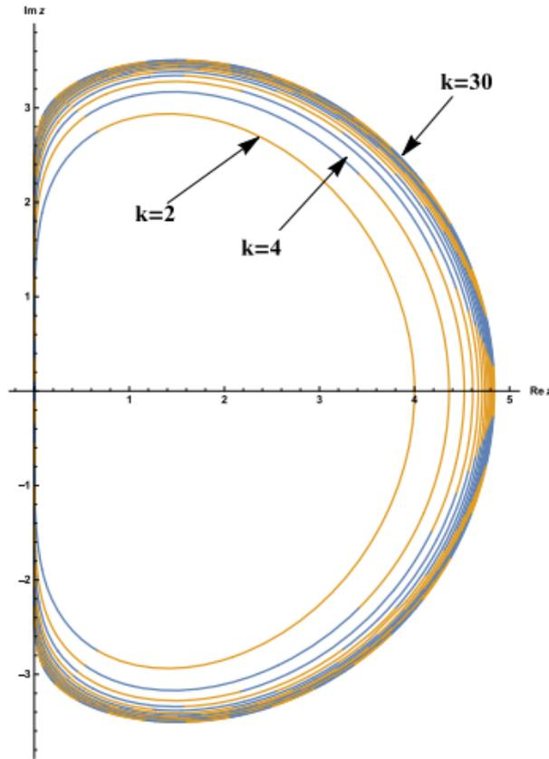
Figure 3: Stability region (exterior of closed curve) of GSDLMME in [28],  $k = 2(2)30$ . The curves are for  $k = 2, 4, 6, 8, \dots, 30$ . However, the curves for  $k = 6, 8, 10, \dots, 30$  are so close to one another that they are indistinguishable.
