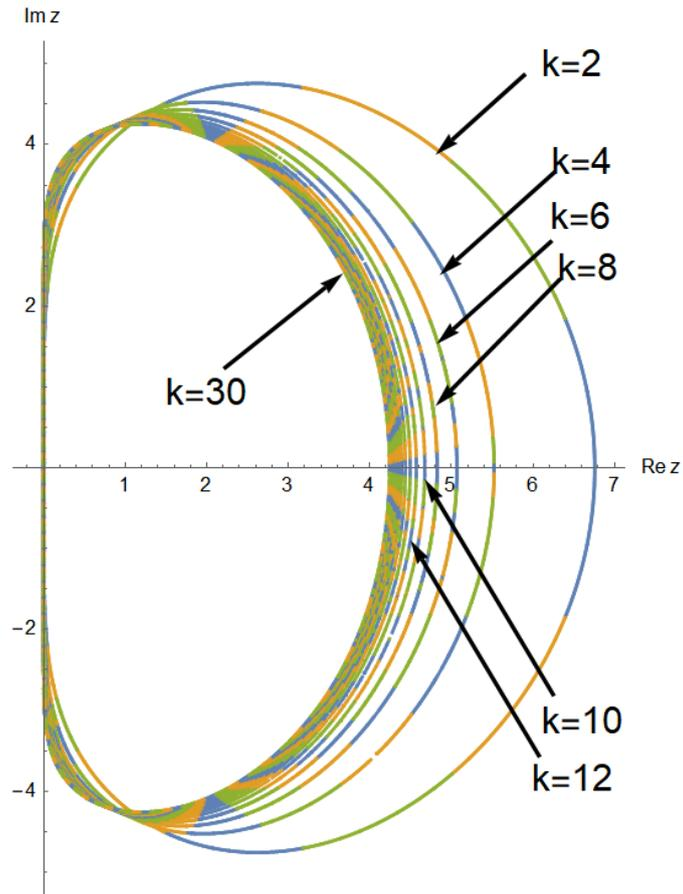
Figure 6: Stability region (exterior of closed curve) of TDGEMs (15),  $k = 2(2)30$ .
