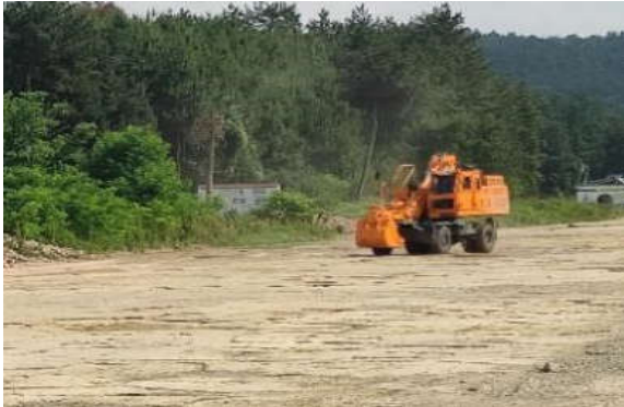
Fig. 6. Experiments of high-speed wheeled excavators driving on uneven roads.
