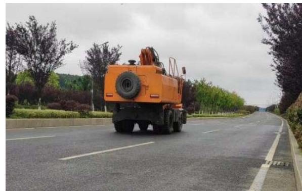
Fig. 10. Experiments of high-speed wheeled excavators driving on uneven roads.
