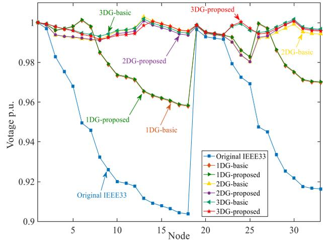
Fig. 7. Node voltage profiles on standard DN with constant loads
