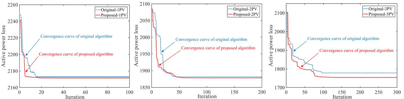
Fig. 9. Convergence curves of practical OAO problems with PV access
