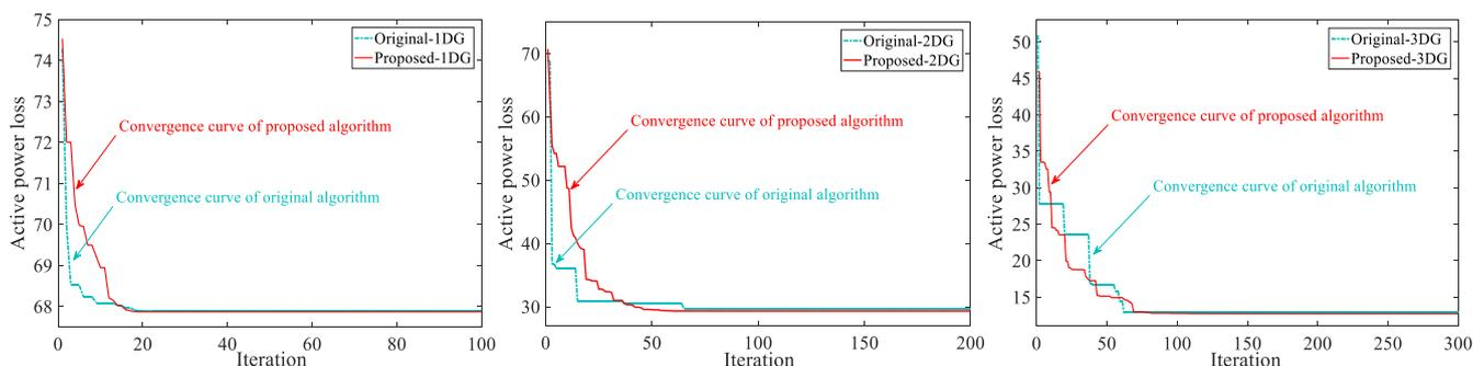
Fig. 6. Convergence curves of BSOA and ISOAE for solving OAO problems with constant loads
