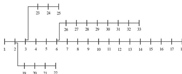
Fig. 3. Single line diagram of IEEE 33-bus system
