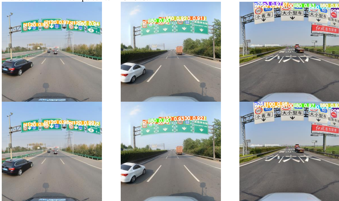
Fig. 9. Comparison of the detection effect of YOLOv8s and the improved YOLOv8s algorithm
