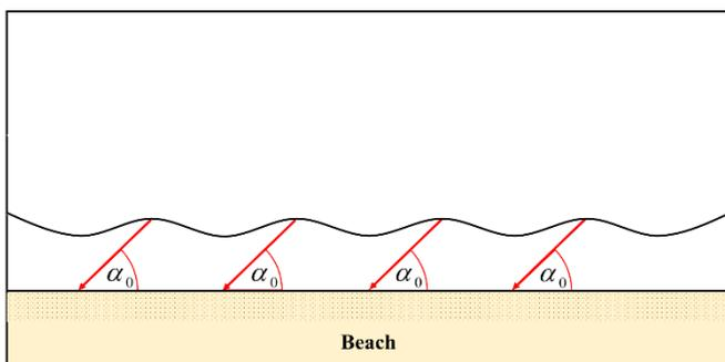
Fig. 3. Breaking wave crests impact angle (the version is redrawn based on [15]).
