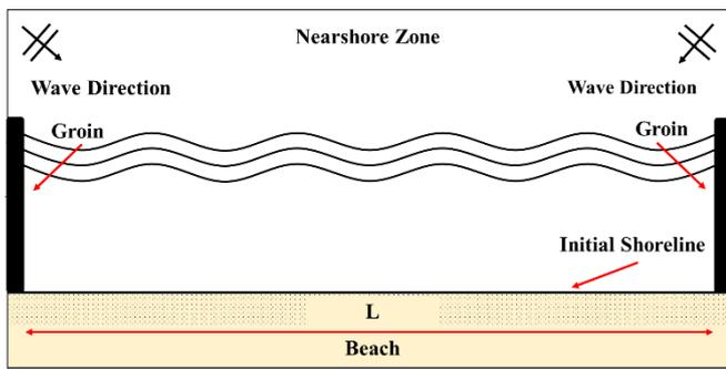
Fig. 1. The shoreline begins with a straight twin groin structure.
