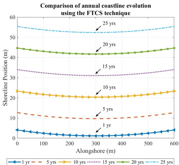
Fig. 12. Comparison of annual shoreline evolution approximated using the FTCS technique.
