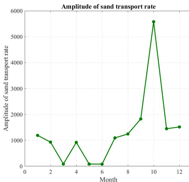
Fig. 5. Amplitude of the long-shore sand transport rate.
