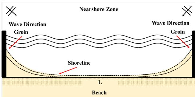
Fig. 2. Shoreline evolution with a straight twin groin structure.
