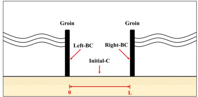
Fig. 4. Setting initial and boundary conditions.
