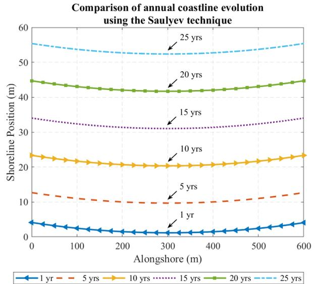
Fig. 13. Comparison of annual shoreline evolution approximated using the Sauljev technique.
