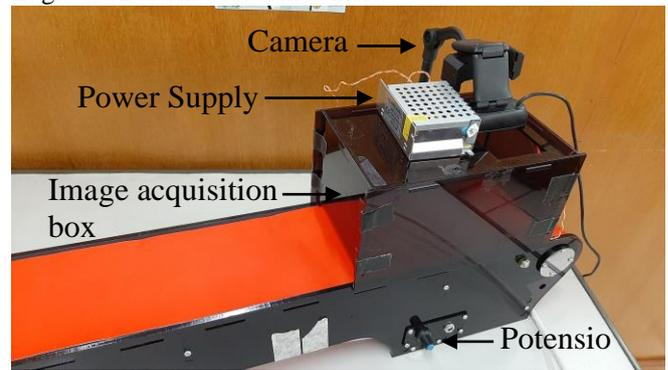
Fig 2. Image Acquisition Prototype with the box panel on the top.
