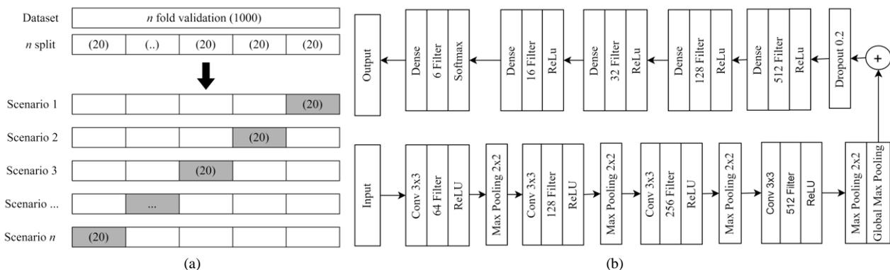
Fig. 5. Diagram of k-fold forward cross-validation (a) & VGG16 block on this research (b)
