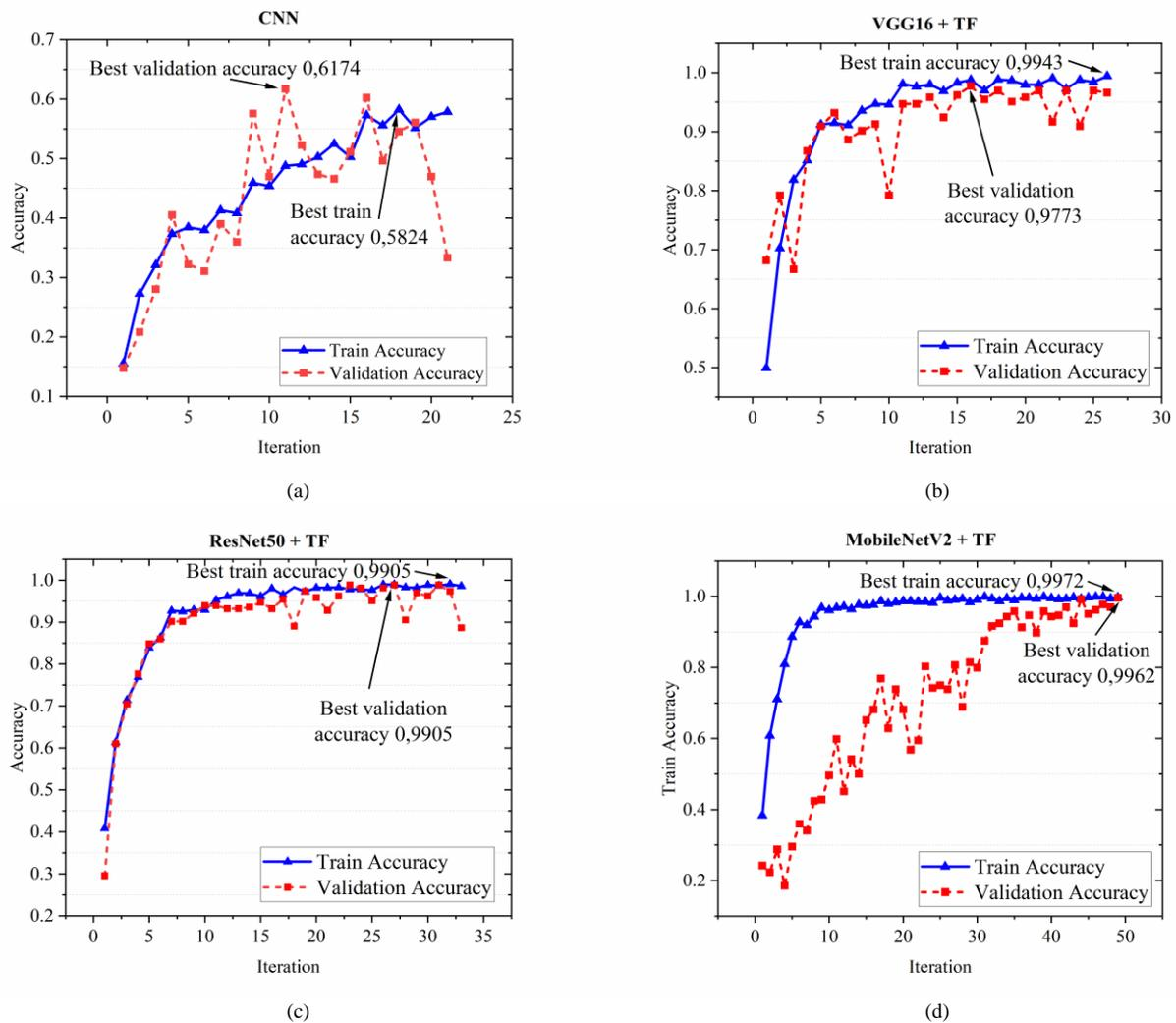
Fig. 7. Performance accuracy of CNN (a), VGG16+TF (b), ResNet50+TF models (c), and MobileNetV2+TF (d)
