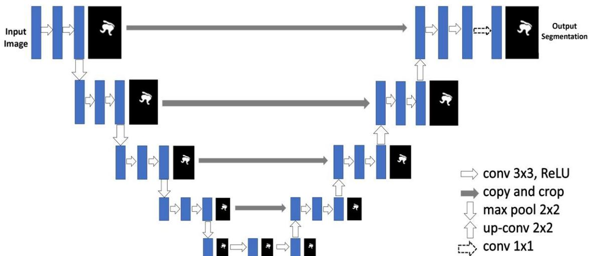
Fig. 1. U-Net architecture with ReLU activation function
