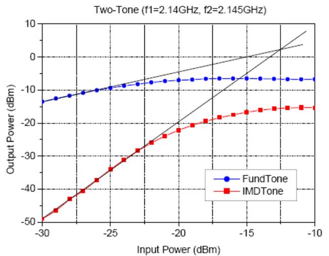
Fig. 10. Measured IIP3 of the LNA.
