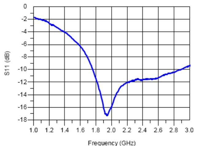
Fig. 5. Measured S11 of the LNA.
