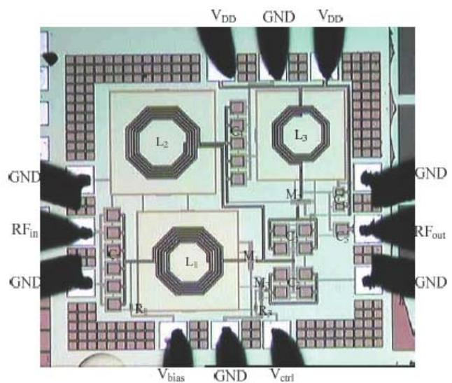
Fig. 4. Microphotograph of the LNA.
