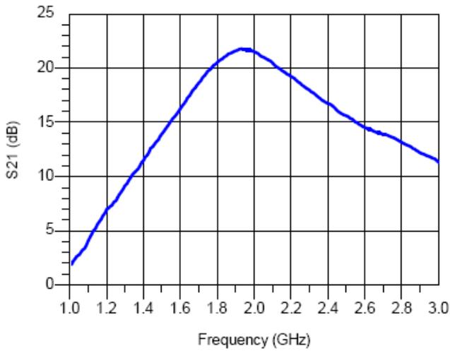
Fig. 7. Measured S21 of the LNA.
