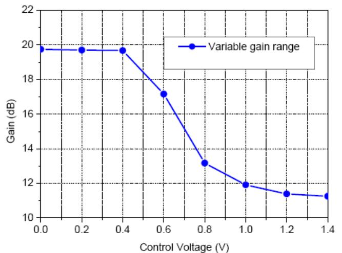
Fig. 11. Measured variable gain range of the LNA.
