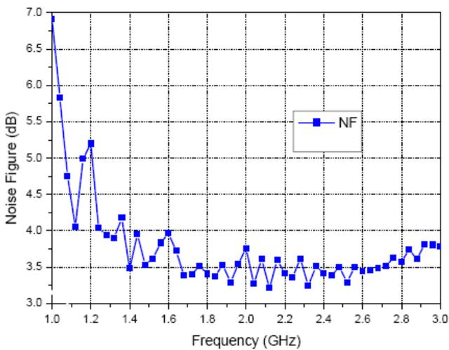
Fig. 8. Measured noise figure of the LNA.
