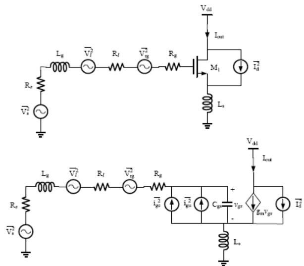
Fig. 1. Equivalent circuit of MOS noise calculation for input stage.
