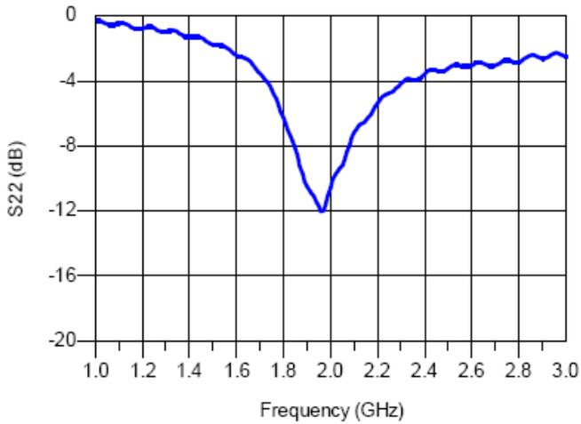
Fig. 6. Measured S22 of the LNA.
