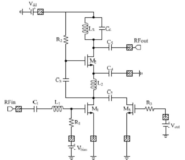
Fig. 2. Designed circuit of the low noise amplifier.
