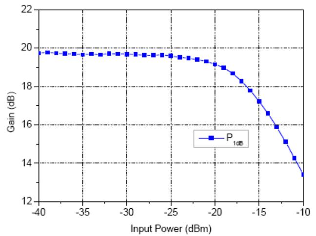
Fig. 9. Measured gain of the LNA.
