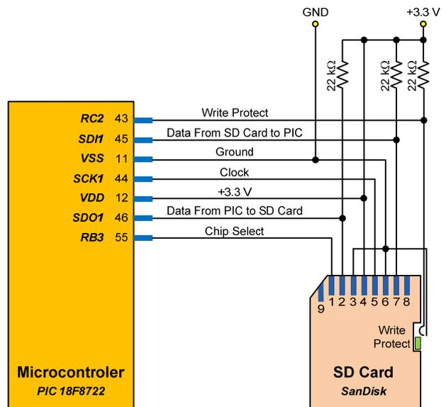
Fig. 15 – Connection diagram between the microcontroller and the SD Card.
