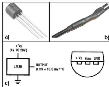
Fig. 3 –Temperature sensor LM35DZ: a) photograph; b) Sensor connected to a cable; c) Pin diagram.
