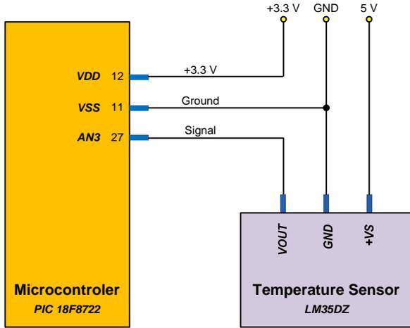
Fig. 4 – Connection diagram between the microcontroller and the temperature sensors. Only one sensor is shown. The other sensors are connected to ports AN4 through AN8 (pins 33, 24, 23, 18 and 17) of the microcontroller instead of port AN3 (pin 27).
