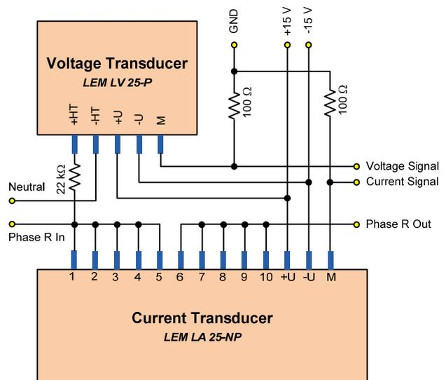
Fig. 8 – Connection diagram of the voltage and current transducers. Only one phase is shown.
