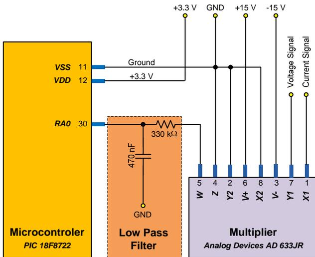
Fig. 10 – Connection diagram between the microcontroller and the multiplier and low pass filter used to determine the active power from two signals proportional to the AC voltage and AC current. Only one phase is shown. The circuits for the other two phases are connected to ports RA1 (pin 29) and RA2 (pin 28) of the microcontroller instead of port RA0 (pin 30).
