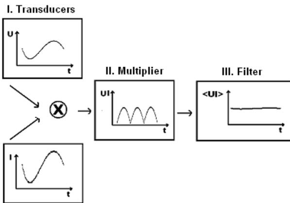
Fig. 5 – Block diagram of the active power measurement circuit.
