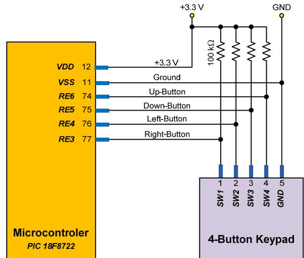
Fig. 18 – Connection diagram between the microcontroller and the 4-button keypad.
