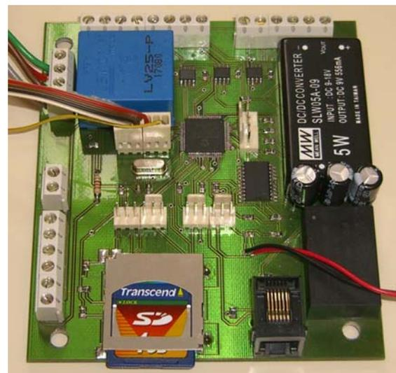
Fig. 19 – Photogram of the main printed circuit board. It contains the storage hardware (SD-Card), the PIC and RTC components, the DC/DC converters and the transducer for the DC voltage analysis from the rectifiers.
