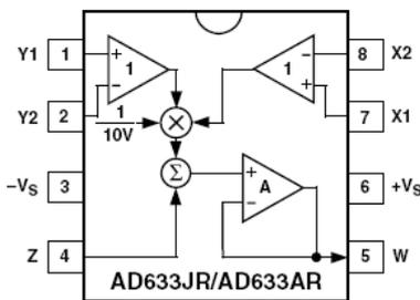
Fig. 9 – Pins of the AD633JRZ multiplier.
