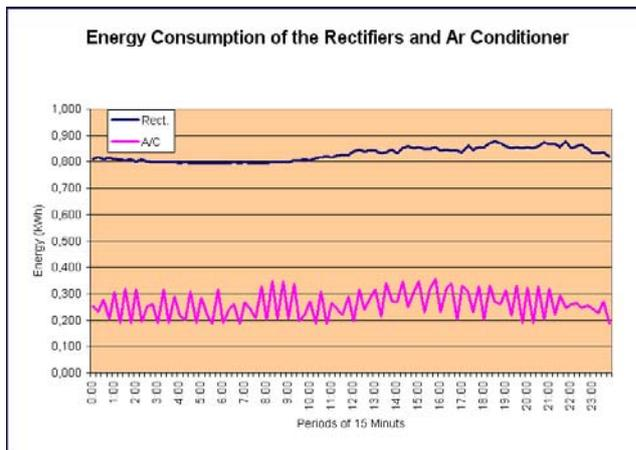
Fig. 21 – Evolution of the total energy consumption of the rectifiers (top) and air conditioning unit (bottom) during one day.
