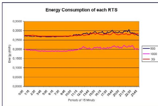
Fig. 22 – Total diary energy consumption of each RBS: GSM900 (top, dark), GSM1800 (bottom) and UMTS/3G (top, light).
