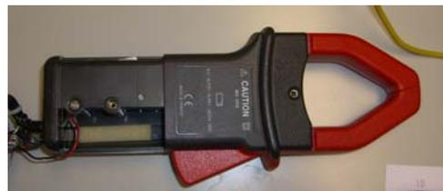
Fig. 12 – Amperimetric Clamp PAC 21 from Chauvin Arnoux.
