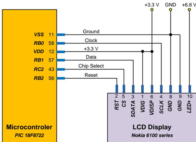
Fig. 17 – Connection diagram between the microcontroller and the LCD display.
