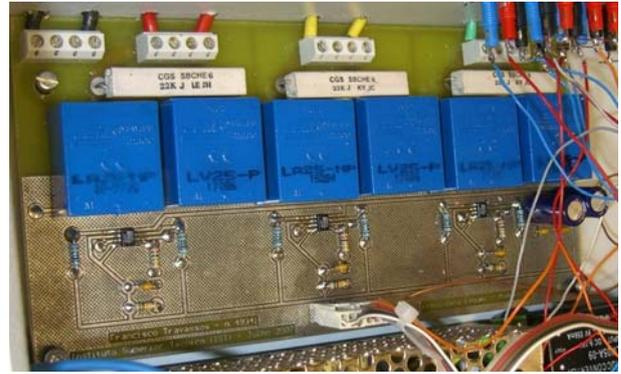
Fig. 11 – Photograph of the three-phase power measurement board.
