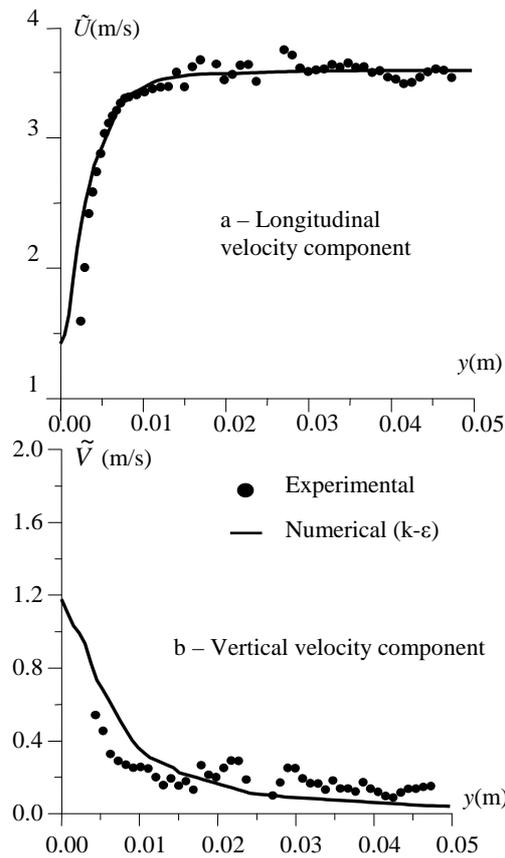
Fig. 2 Confrontation of the longitudinal and vertical velocity distributions in the symmetry plane, within the upstream jet location ( $x=0$  mm)
