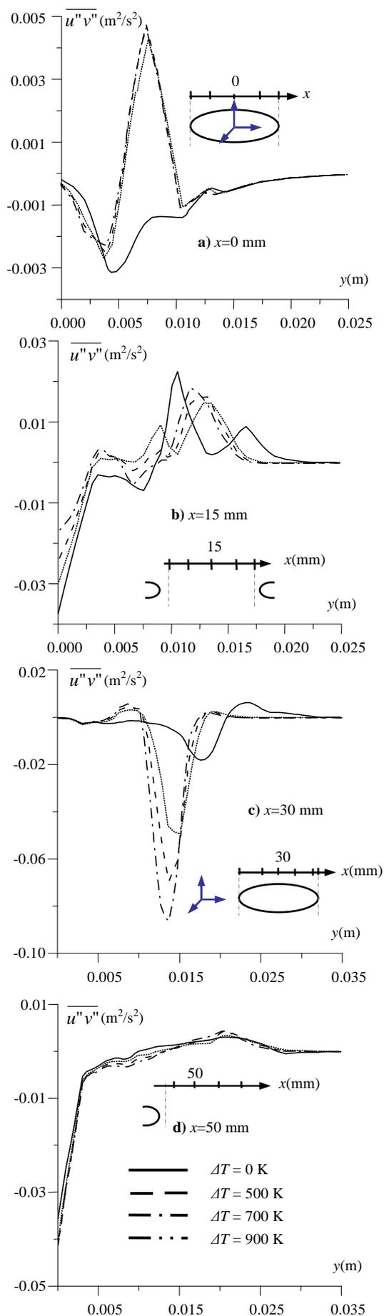
Fig. 3 Impact of the temperature gradient on the vertical distribution of the tangential  $u''v''$  shear stress component
