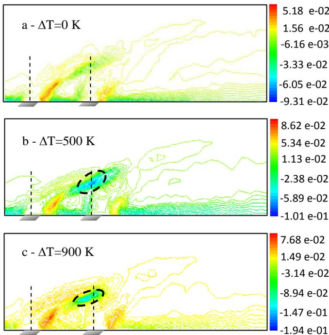
Fig. 4 Contours of the  $\overline{u'v'}$  ( $\text{m}^2/\text{s}^2$ ) shear stress component on the symmetry plane under the isotherm,  $\Delta T=500$  K and  $\Delta T=900$  K cases
