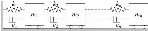
Figure 3: Mechanical model of the linear 1-D structure.
