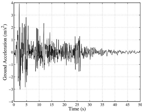
Figure 9: El-Centro Earthquake scaled to  $0.4g$  (NS components).
