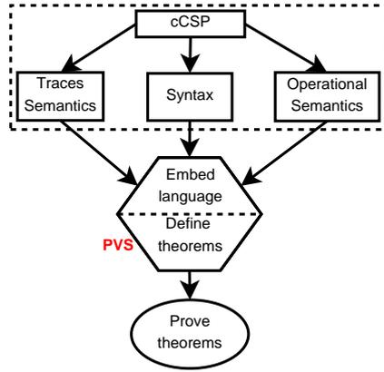
Figure 7: PVS mechanization steps
