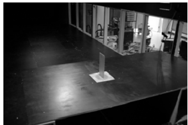
Figure 6 – Pressure tapped wing - 3-D configuration mounted on ground plane, RMIT IWT
