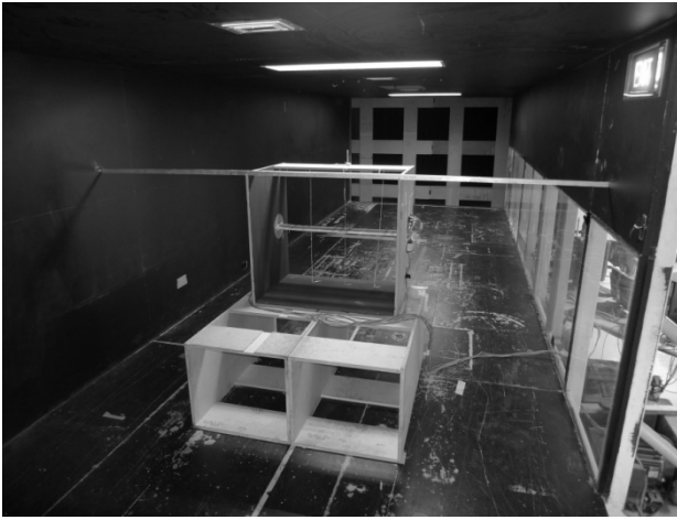
Figure 4 – Pressure tapped wing - 2-D configuration between end plates RMIT IWT
