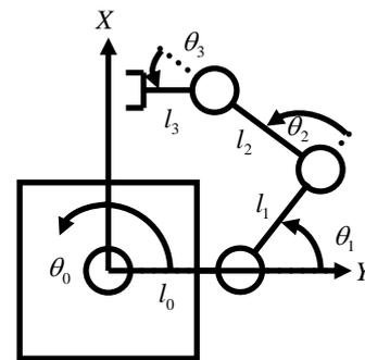
Fig.1 Model of Space Robot
