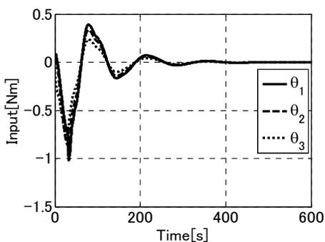
Fig.19 History of Torque Control Input
