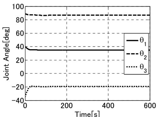
Fig.16 History of Joint Angles for Space Robot
