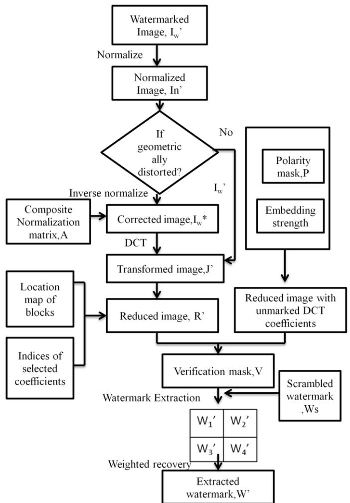
Fig. 6. Watermark detection scheme
