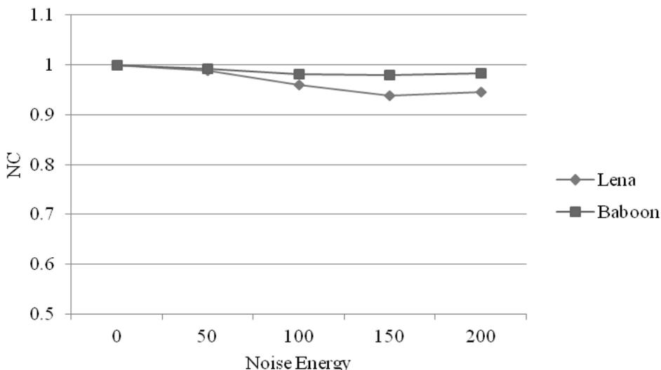
**Fig. 14.** Performance of FGRW scheme against additive noise attack
