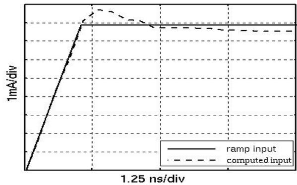
Fig. 3. Waveform of the injected current used for simulation.
