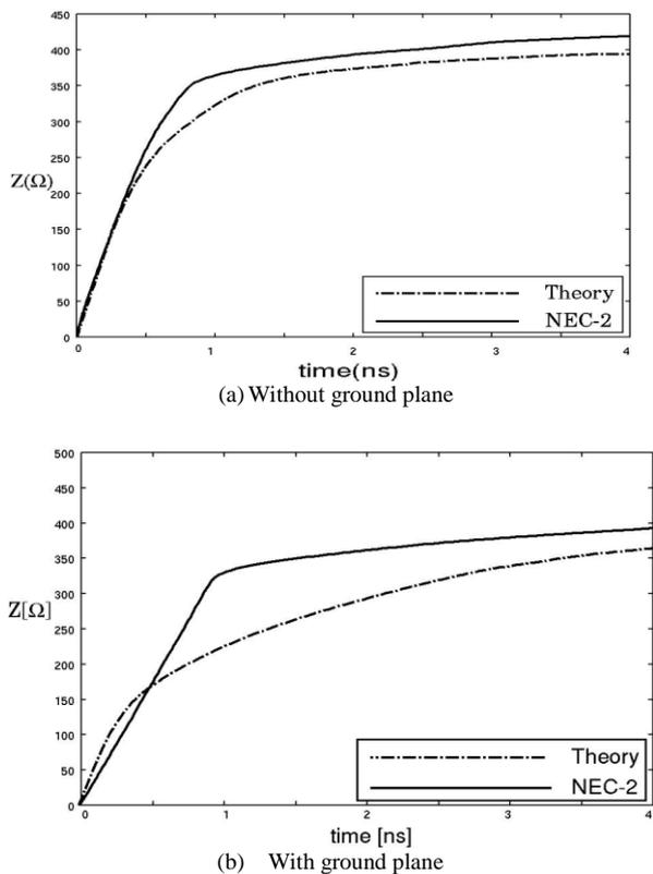
Fig. 7. Surge impedance of the vertical conductor of 60 cm at  $0 < t \leq 2h/c$ .
