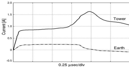
(b) Current in the tower and earth wire due to stroke to mid-span
