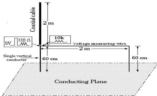
Fig. 2. Arrangement of the vertical conductor system for the simulation with NEC-2 without ground plane.
