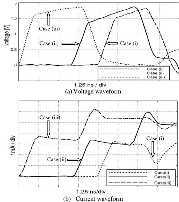
Fig. 15. Computed waveforms of voltage and currents for injection at different height of the current lead wire.
