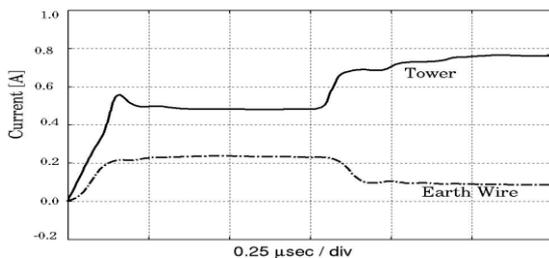
(b) Current in the tower and earth wire due to return stroke to the tower
