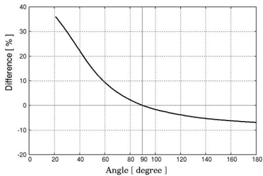
(b) Effect of the angle between current lead wire and voltage measuring wire.
