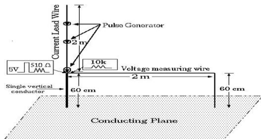
Fig. 14. Arrangement for the analysis by the direct method, where a pulse generator is placed at different position in the current lead wire.
