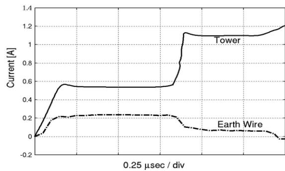
Fig. 22. Computed waveforms of current splitting ratio into the tower and earth wire due to downward travelling current to the tower.
