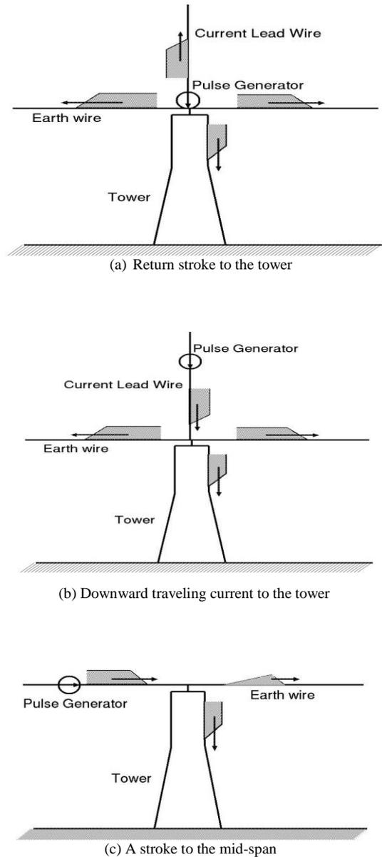
Fig. 19. Schematic diagrams for simulation of current splitting ratio between a tower and earth wire
