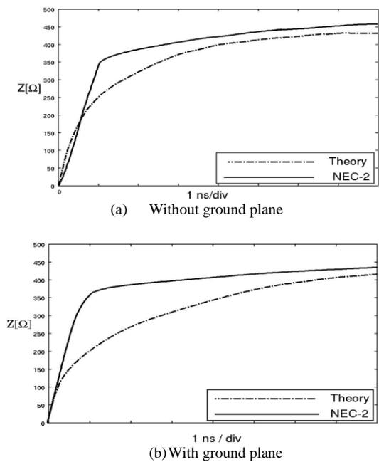
Fig. 13. Surge impedance of the vertical conductor of 120 cm at  $0 < t \leq 2h/c$ .
