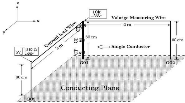
Fig. 1. Arrangement of the vertical conductor system for the simulation with NEC-2 with ground plane.
