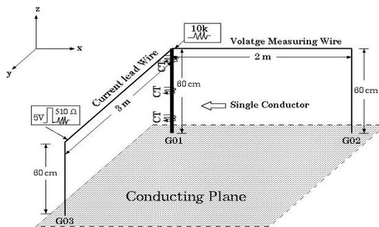
Fig. 1. Arrangement of the vertical conductor system for the simulation with NEC-2 with ground plane.
