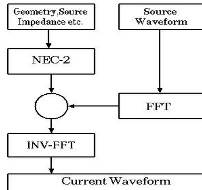
Fig. 4. Flowchart of the solution using NEC-2.
