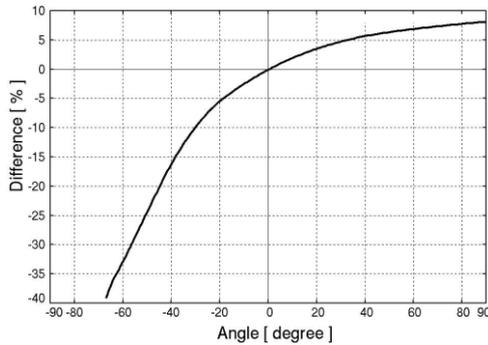
(a) Effect of the angle between current lead wire and voltage measuring wire.
