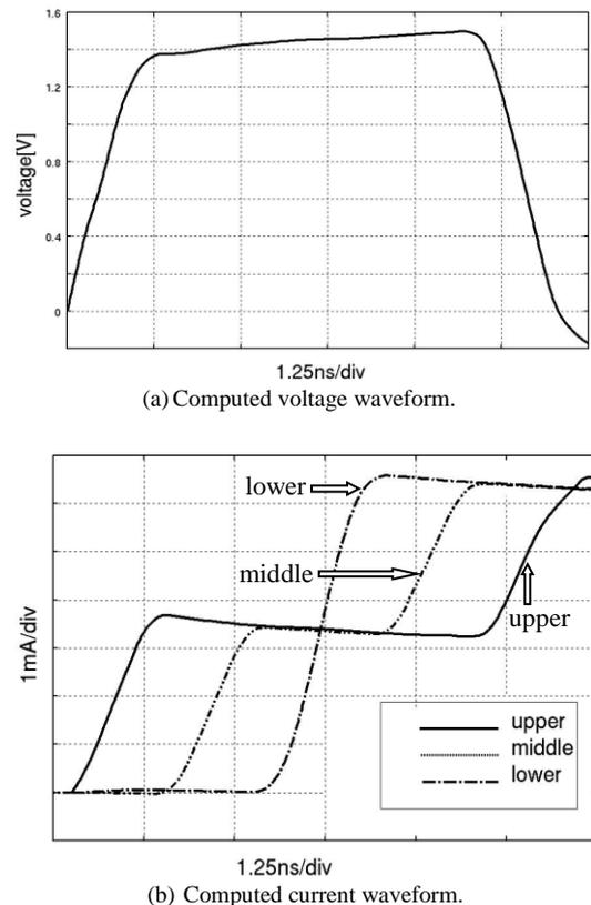
Fig. 8. NEC-2 results of voltage at the top and currents through the vertical conductor of 90 cm in case without ground plane.
