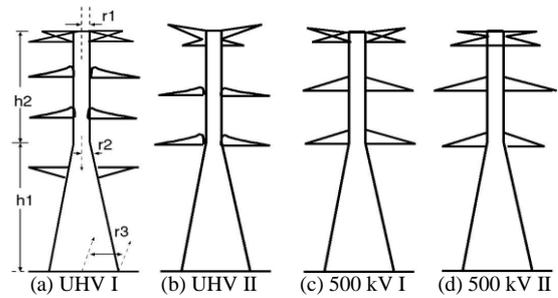
Fig. 24. Structures of 1000 kV and 500 kV double circuit towers.
