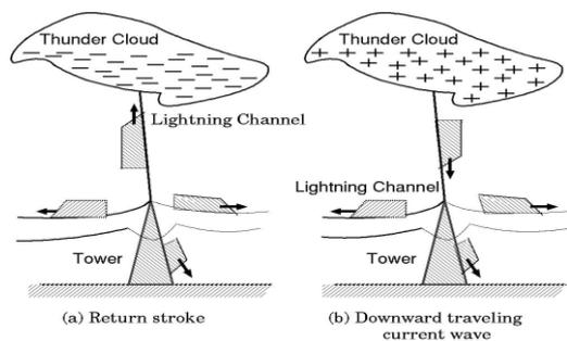
Fig. 16. Schematic diagrams of different types of lightning strokes to the top of a tower.
