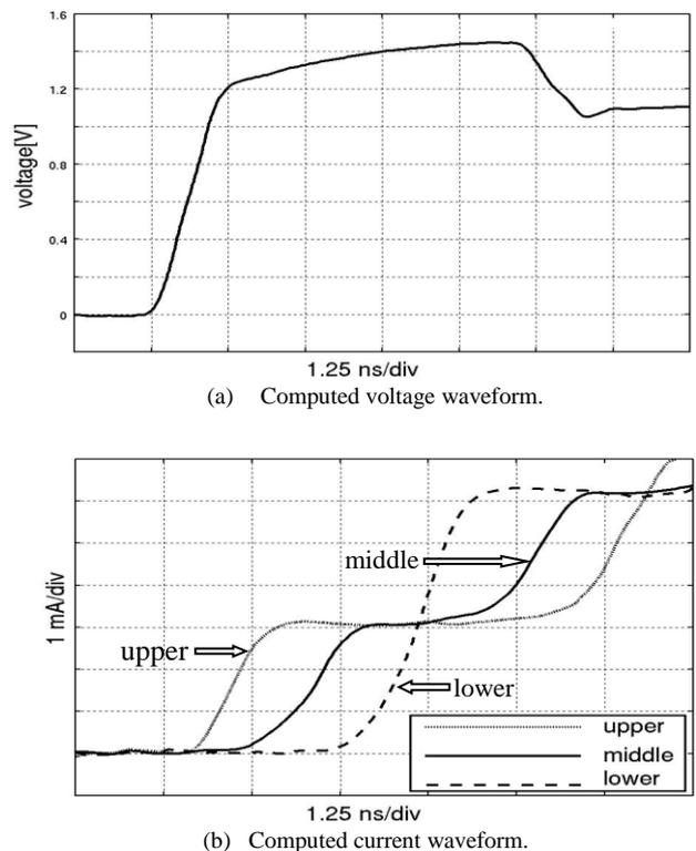
Fig. 9. NEC-2 results of voltage at the top and currents through the vertical conductor of 90 cm in case with ground plane.
