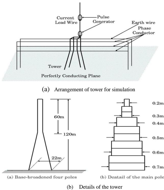
Fig. 17. The structure of the model tower subjected to analysis.
