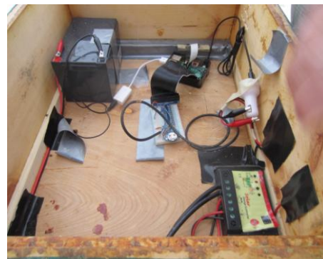
Fig. 1. BeePi hardware components.
