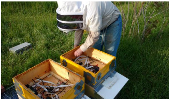
Fig. 5. Wiring BeePi monitors for deployment .
