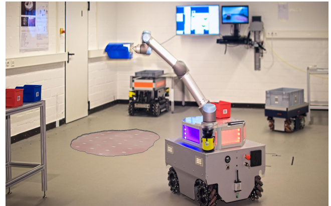
Fig. 1. Floor installed RFID tags for localization of mobile robots
