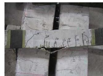
Fig.8 Crack distribution of No.1 beam
