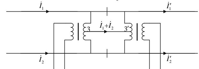
Fig. 5. Diagram of the Working Principle of the Choke Transformer
