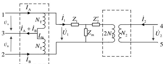
Fig. 7. Equivalent Circuit of the Choke Transformer
