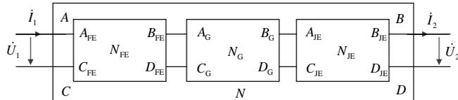
Fig. 9. Cascade Adjustment Mode Choke Transformer and the Track Circuit's Four-terminal Network
