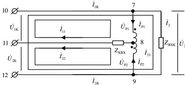
Fig. 4 Equivalent Circuit of the Receiving Terminal of Track Circuit
