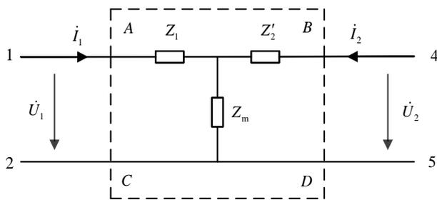
Fig. 6. T-type Equivalent Circuit of Choke Transformer
