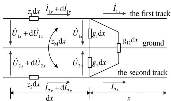
Fig. 1. Equivalent Circuit of Short  $dx$  for Track Line
