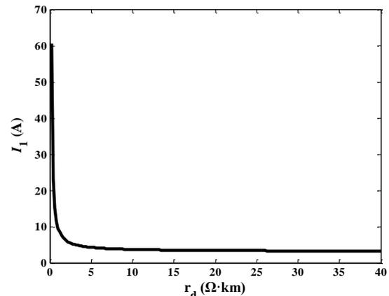
Fig. 13. Change in the Sending Terminal Current with Ballast Resistance
