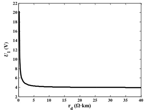
Fig. 12. Change in the Sending Terminal Voltage with Ballast Resistance
