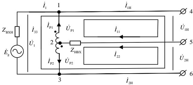
Fig. 3 Equivalent Circuit of the Power Supply Terminal of Track Circuit
