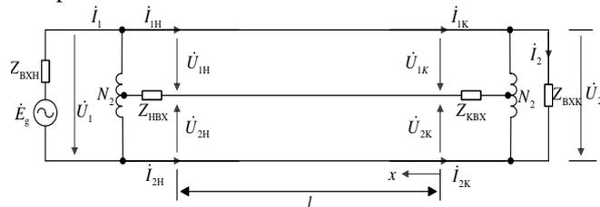
Fig. 2. Equivalent Circuit of the Four-terminal Network of the Track Circuit
