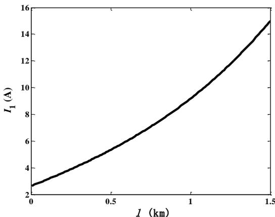
Fig. 11. Change in the Sending Terminal Current with Transmission Distance
