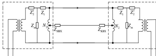
Fig. 8. Equivalent Circuit of the Adjustment Mode Choke Transformer Combined with Track Circuit
