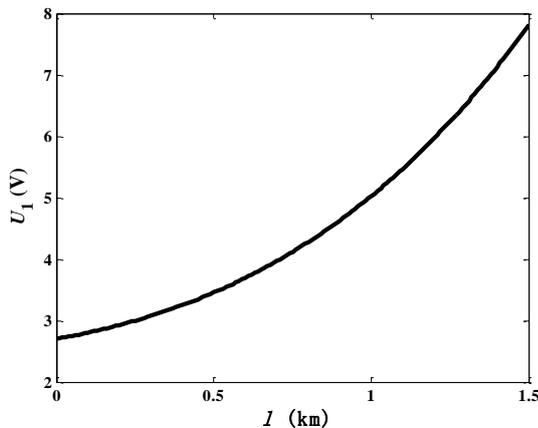
Fig. 10. Change in the Sending Terminal Voltage with Transmission Distance
