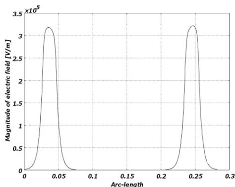
Fig. 11. Electric field and potential distributions on hydrophilic and polluted insulator surface with lower-upper dry-bands by applying  $v_{2x}$  ; inside the insulator core path
