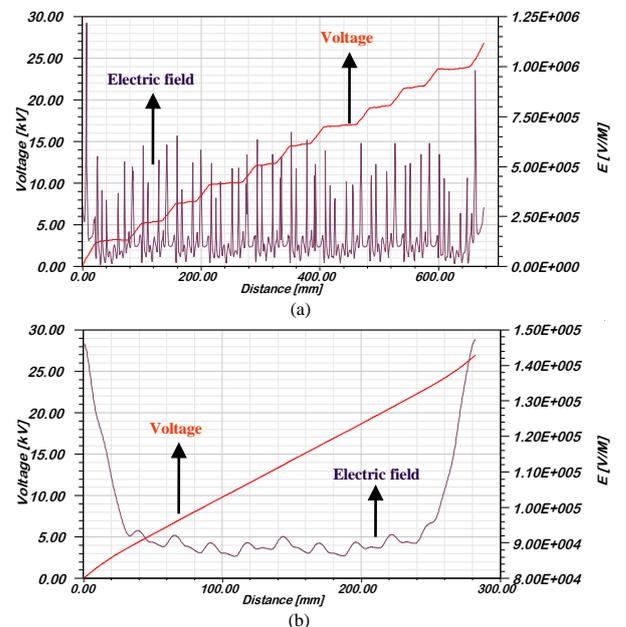
Fig. 3. Electric field and potential distributions on hydrophobic and polluted surface insulator condition, and without dry-band, by applying  $v_{1x}$ ; (a) along creepage path, (b) inside the insulator core
