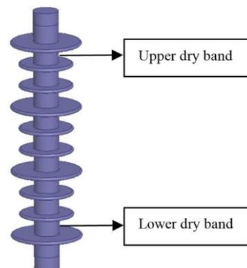
Fig. 1. Structure of composite insulator with dry-bands location.
