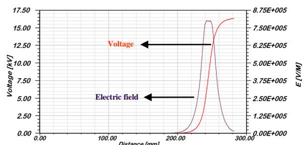
Fig. 9. Electric field and potential distributions in the hydrophilic state with lower dry-band and with the length of 10 mm in voltage level  $v_{2x}$  , inside the insulator core
