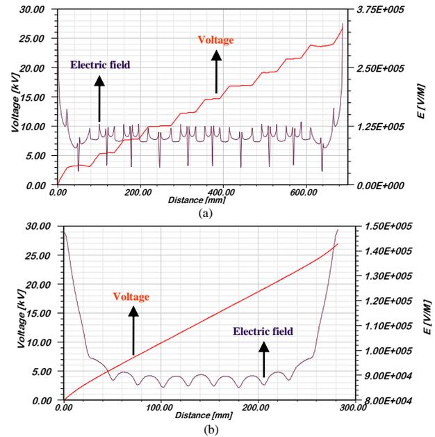
Fig. 2. Electric field and potential distributions on clean and dry insulator by applying  $v_{1x}$ ; (a) along the creepage path, (b) inside the insulator core
