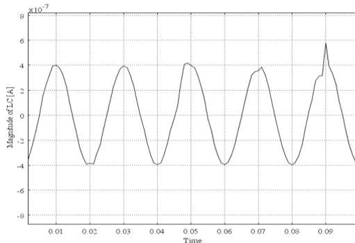
Fig. 11 .The leakage current of clean and dry insulator by applying  $v_{1x}$
