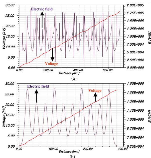
Fig. 5. Electric field and potential distributions on hydrophilic and polluted surface insulator condition without dry-band and by applying  $v_{1x}$  ; (a) along creepage path , (b) inside the insulator core
