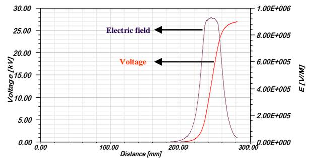
Fig. 6 Electric field and potential distributions on hydrophilic and polluted surface insulator condition with lower dry-band, with applying  $v_{1x}$  ; inside the insulator core
