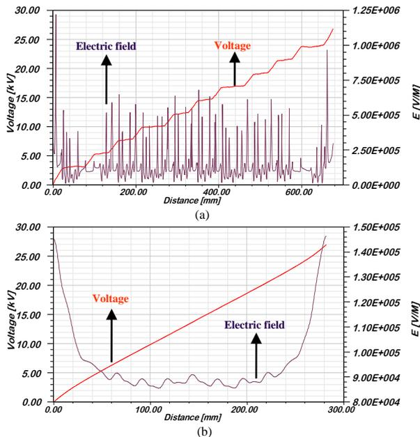
Fig. 4. Electric field and potential distributions on hydrophobic and polluted surface insulator condition, and with lower-upper dry-bands, by applying  $v_{1x}$  ; (a) along creepage path , (b) inside the insulator core
