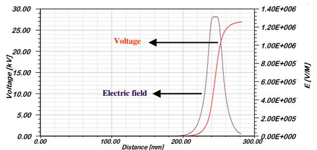
Fig. 8. Electric field and potential distributions in the hydrophilic state with lower dry-band and with the length of 10 mm in voltage level  $v_{1x}$  , inside the insulator core
