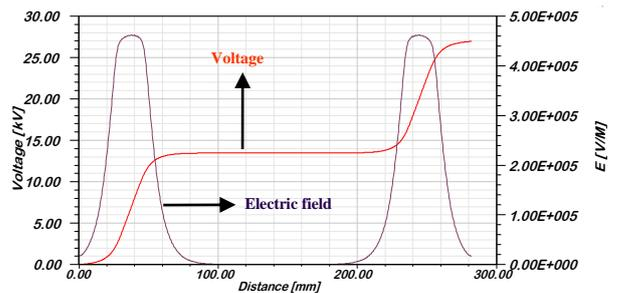
Fig. 7. Electric field and potential distributions on hydrophilic and polluted surface insulator condition with lower-upper dry-bands, by applying  $v_{1x}$  ; inside the insulator core
