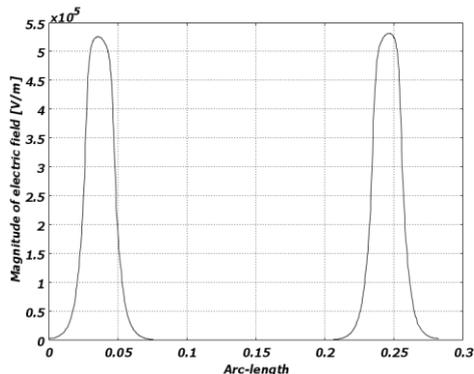
Fig. 10. Electric field and potential distributions on hydrophilic and polluted insulator surface with lower-upper dry-bands by applying  $v_{1x}$  ; inside the insulator core path
