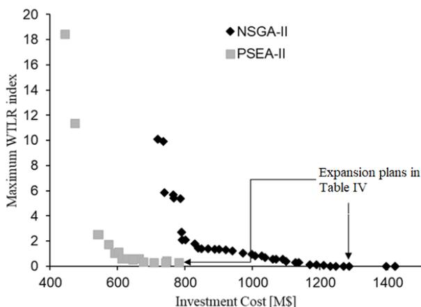
Fig. 9. Pareto fronts obtained with the NSGA-II and the PSEA-II in Scenario 1.
