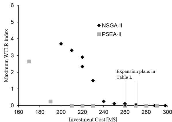
Fig. 4. Pareto fronts obtained with the NSGA-II and the PESA-II in Scenario 1.
