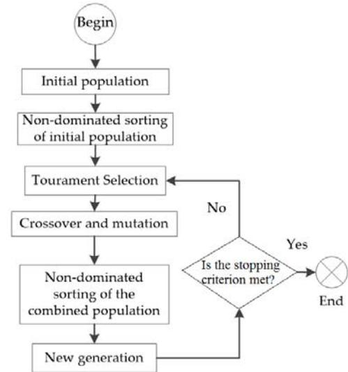
Fig. 2. Flowchart of the NSGA-II implemented in this work.
