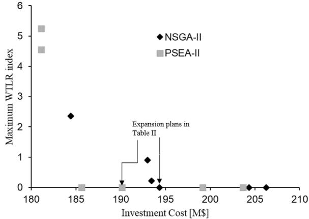
Fig. 5. Pareto fronts obtained with the NSGA-II and the PSEA-II in Scenario 2.
