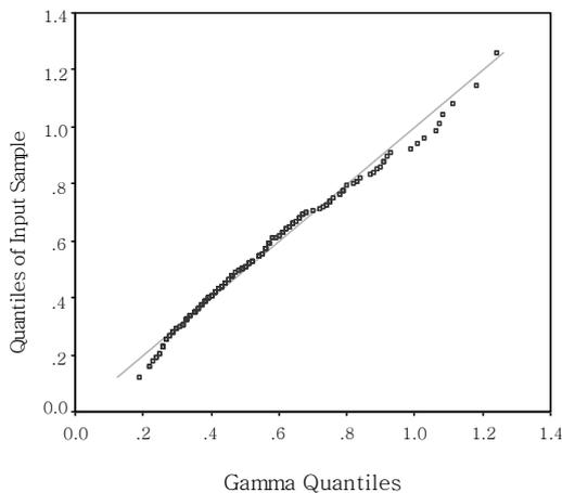
Fig 1 The Gamma probability plots for the degradation data
