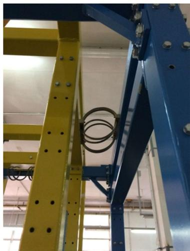
Fig. 26. Wire rope spring stabilizers
