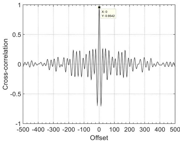
Fig. 2. Cross-correlation function of explosion seismic waves
