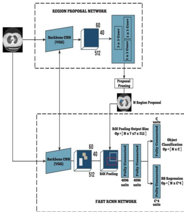
Fig. 5. The Faster-RCNNs architecture.
