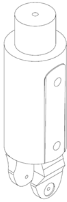
Fig. 11. The Design of the Double Cutter Actuator
