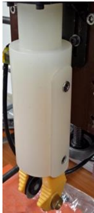
Fig. 12. The Fabricated Double Cutter Actuator
