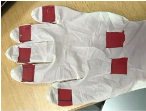
Fig. 21. Sample glove after Cutting Test are performed
