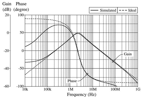
Fig. 5. Ideal and simulated frequency characteristics of the BP filter obtained from Fig.2.
