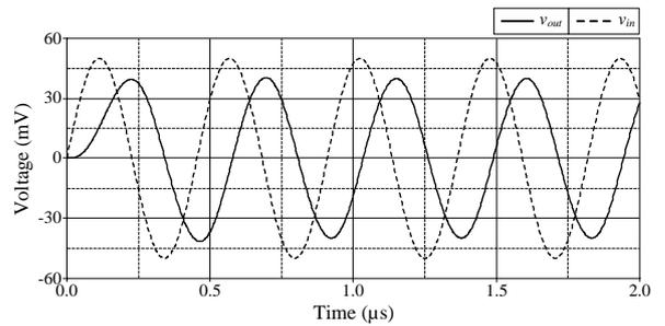
Fig. 9. Simulated time-domain responses of the LP filter of Fig.2.
