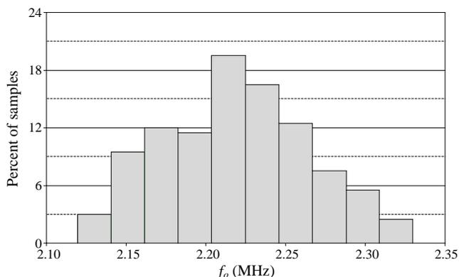
Fig. 17. Monte Carlo statistical analysis of BP response with 5% deviation in capacitances  $C_1$  and  $C_2$  (sample = 200, mean =  $2.21945 \text{ MHz}$ , median =  $2.22201 \text{ MHz}$ , minimum =  $2.11940 \text{ MHz}$ , maximum =  $2.32989 \text{ MHz}$ , sigma =  $45.7446 \text{ kHz}$ ).
