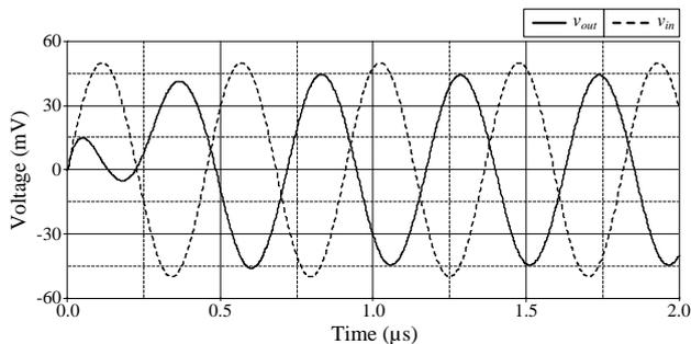
Fig. 13. Simulated time-domain responses of the AP filter of Fig.2.
