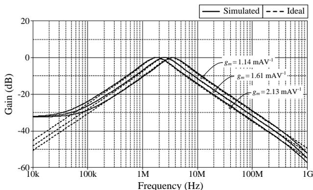
Fig. 14. Electronic  $Q$  tunability of BP response for the proposed filter.
