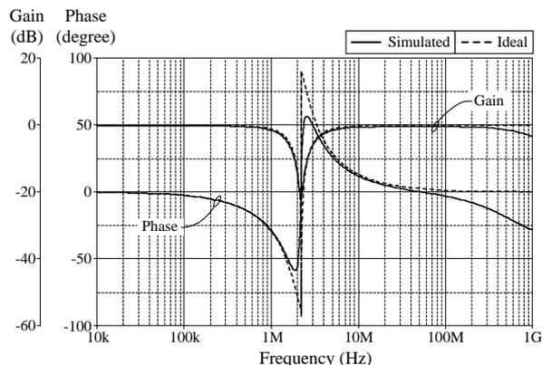
Fig. 7. Ideal and simulated frequency characteristics of the BS filter obtained from Fig.2.
