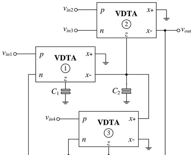
Fig. 2. Proposed VDTA-based universal biquadratic filter
