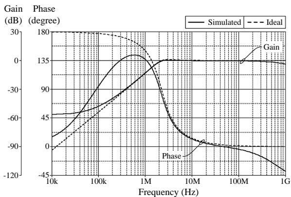
Fig. 6. Ideal and simulated frequency characteristics of the HP filter obtained from Fig.2.
