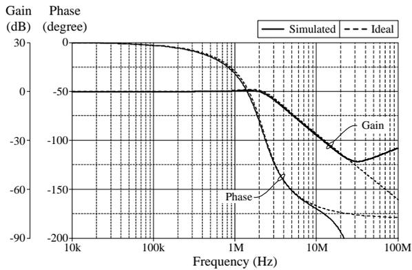
Fig. 4. Ideal and simulated frequency characteristics of the LP filter obtained from Fig.2.
