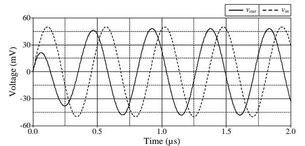
Fig. 11. Simulated time-domain responses of the HP filter of Fig.2.
