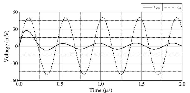
Fig. 12. Simulated time-domain responses of the BS filter of Fig.2.
