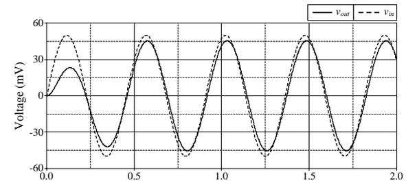
Fig. 10. Simulated time-domain responses of the BP filter of Fig.2.
