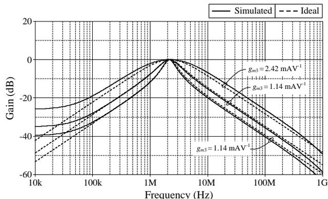
Fig. 15. Electronic  $f_o$  tunability of BP response for the proposed filter.
