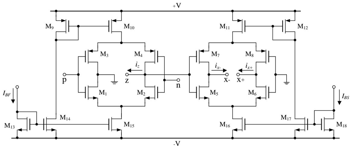
Fig. 3. CMOS realization of the VDTA
