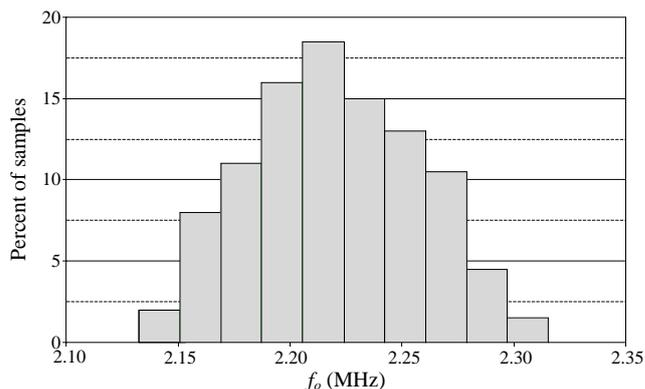
Fig. 16. Monte Carlo statistical analysis of BP response with 5% deviation in transconductances  $g_{mFi}$  and  $g_{mSi}$  (sample = 200, mean =  $2.21955 \text{ MHz}$ , median =  $2.21703 \text{ MHz}$ , minimum =  $2.13252 \text{ MHz}$ , maximum =  $2.31543 \text{ MHz}$ , sigma =  $37.9206 \text{ kHz}$ ).
