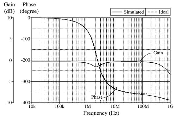
Fig. 8. Ideal and simulated frequency characteristics of the AP filter obtained from Fig.2.
