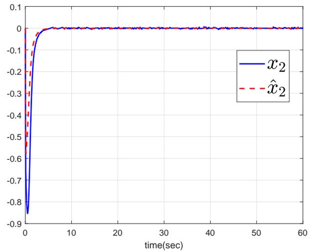
Fig. 2. The states of  $x_2$  and  $\hat{x}_2$  in fault-free situation
