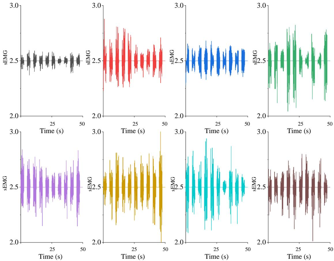
FIGURE 5. The following signals were acquired during the experiment: (1) sEMG of extensor carpi radialis, (2) sEMG of extensor carpi ulnaris, (3) sEMG of short extensor pollicis, and (4) sEMG of extensor digitorum communis for finger movements; (5) sEMG of carpi radialis, (6) sEMG of extensor carpi ulnaris, (7) sEMG of biceps brachii, and (8) sEMG of triceps for arm movements.
