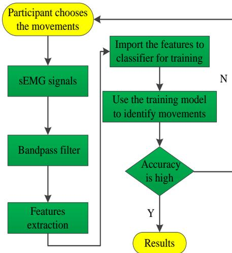
FIGURE 3. The recognition process
