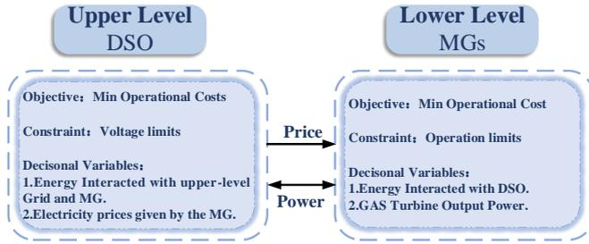
Fig. 2. Coordinated Optimization Framework Based on Multi-Entity.
