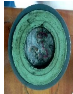
(c) Concrete specimen fixed within the permeability cell.
