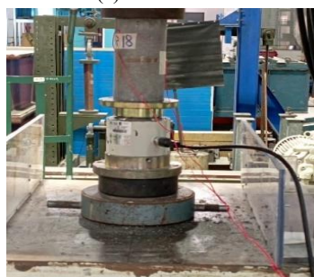
(b) Strain gauges, sample fixation, steel load plates and the loading cell
