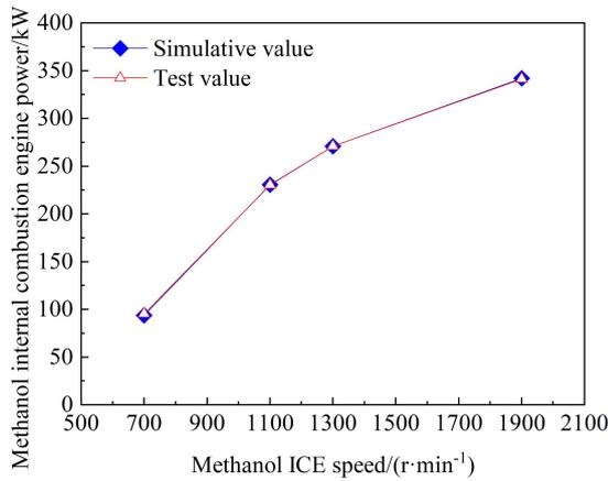
Fig. 3. Typical characteristic speed power calibration of one-dimensional thermodynamic model
