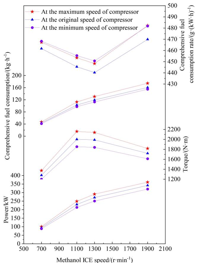
Fig. 12. Influences of maximum and minimum speeds of the compressor on the external characteristics of the methanol ICE
