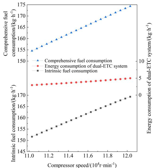
Fig. 9. The influences of the compressor speed on the energy consumption of methanol ICE at 1900rpm
