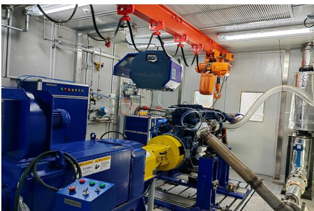
Fig. 2. Methanol ICE test platform
