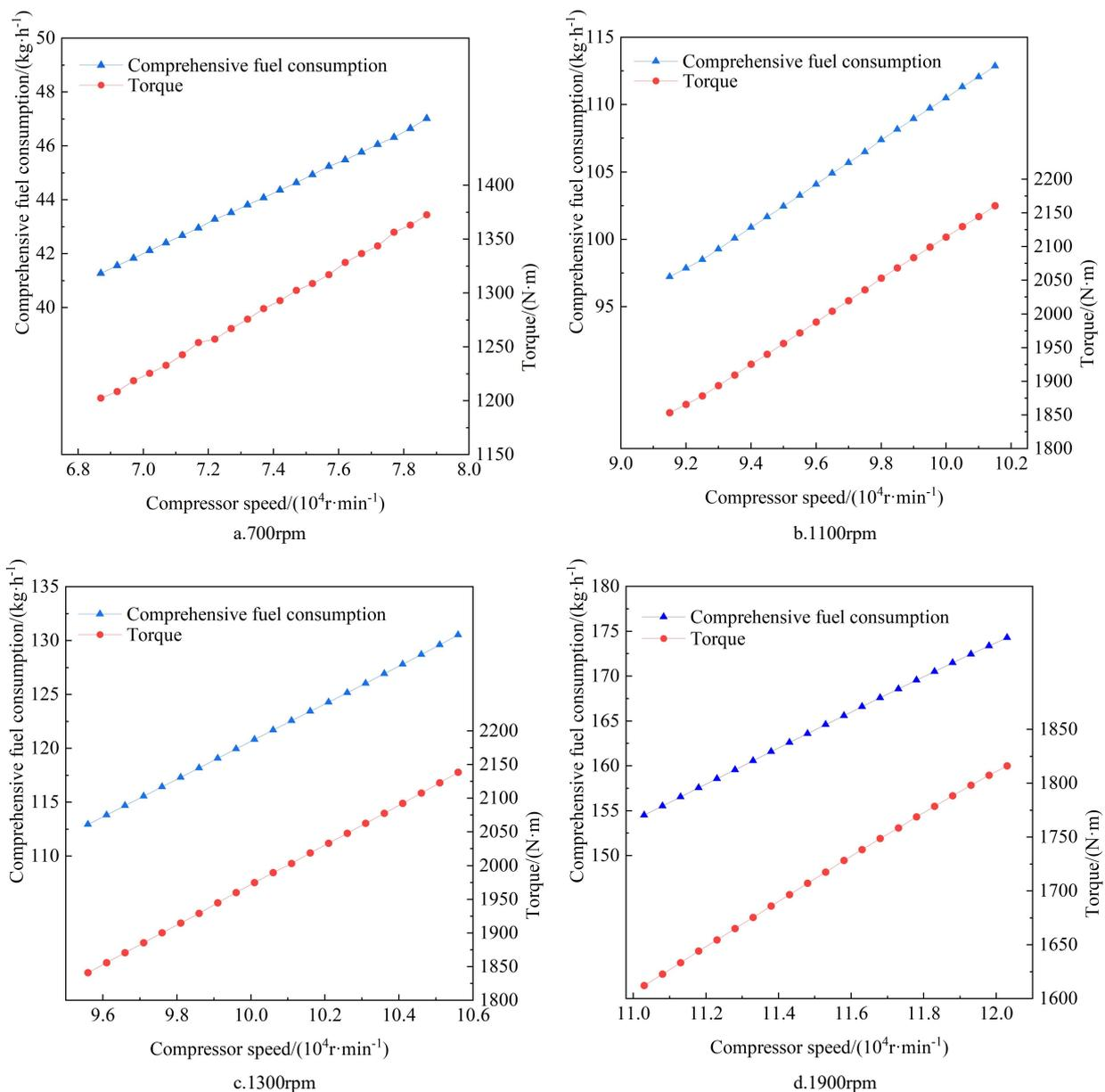
Fig. 11. Relationship between the torque and the comprehensive fuel consumption at each typical characteristic speed conditions of the methanol ICE
