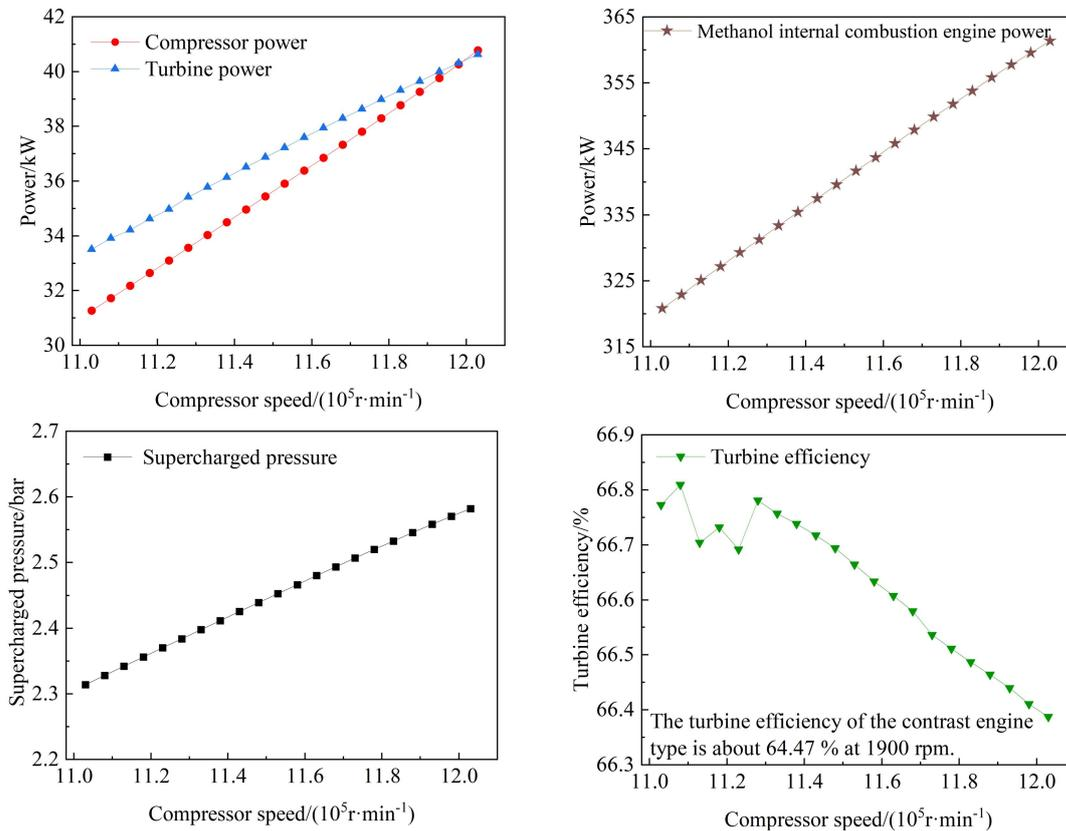
Fig. 8. The influences of the compressor speed on the main performance of the methanol ICE at 1900rpm
