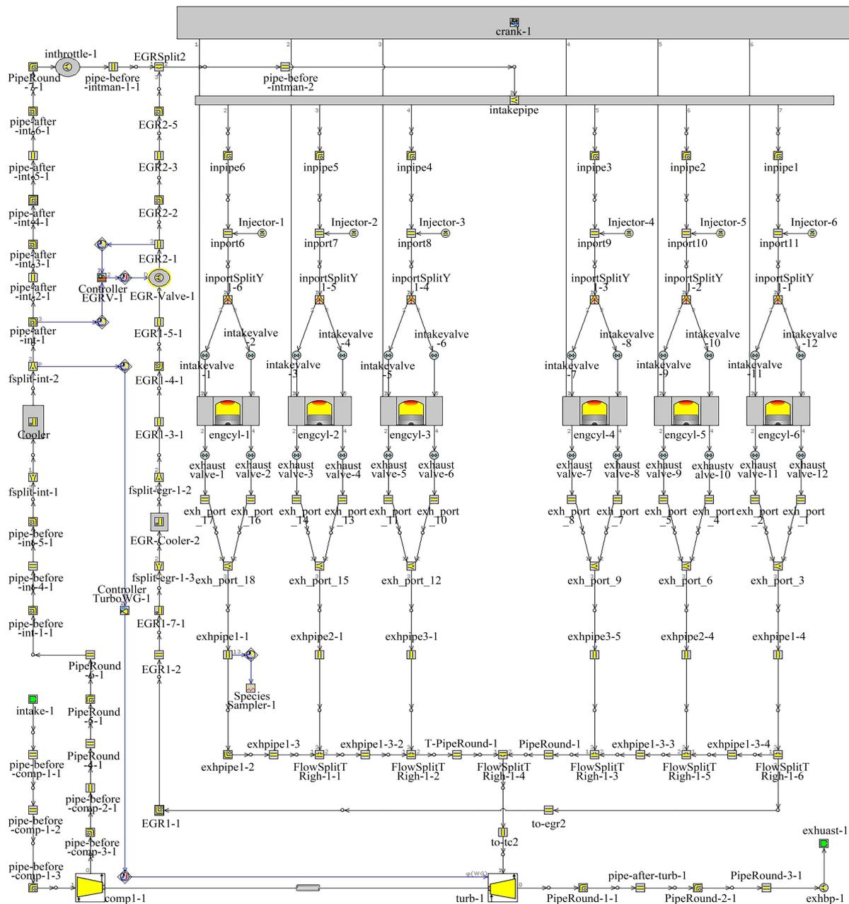
Fig. 1. One-dimensional thermodynamic simulation model of methanol ICE
