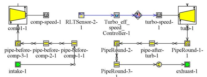
Fig. 5. Simulation model of the dual-ETC system
