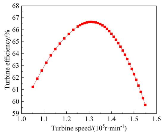
Fig. 7. The change relationship between the turbine speed and efficiency
