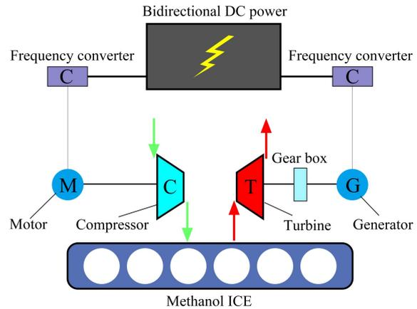
Fig. 6. Working principle diagram of the dual-ETC system for the methanol ICE
