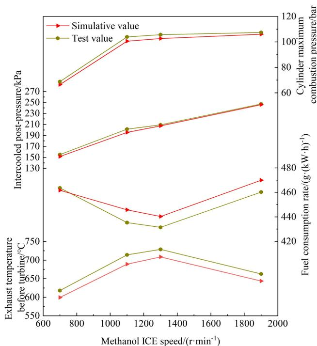
Fig. 4. Comparison of experimental value and simulation value of one-dimensional thermodynamic model
