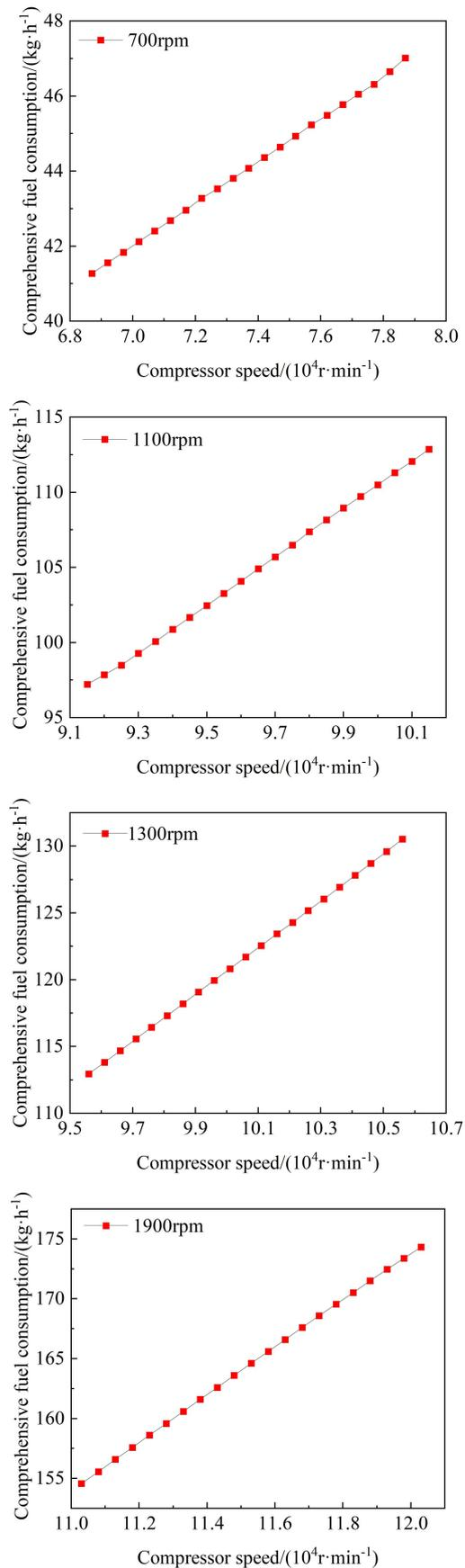
Fig. 10. The influences of the compressor speed on comprehensive fuel consumption under the typical characteristic speed conditions of the methanol ICE
