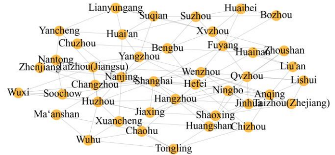
Fig. 6. Topology diagram of the hyperedge relationship of the comprehensive transportation supernetwork
