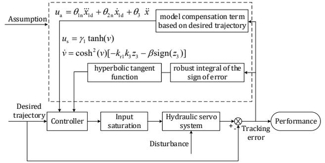
Fig. 2. Structure of the proposed controller
