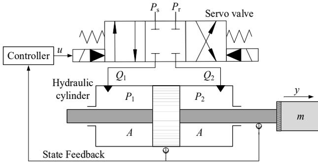
Fig. 1. Structure of considered hydraulic servo system
