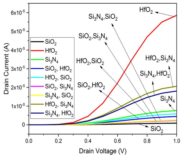
Fig. 6:  $I_d - V_{ds}$  for different dielectric materials
