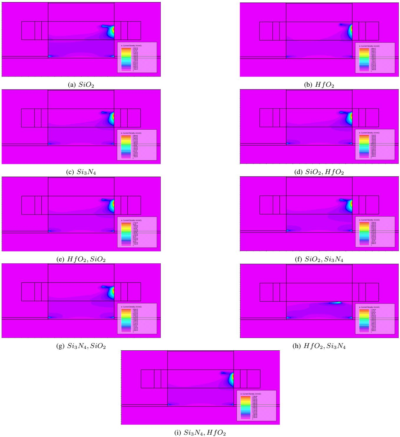
Fig. 12: Electron current density distribution for different dielectric materials, comparing the gate control and carrier transport across the proposed TFET structure.
