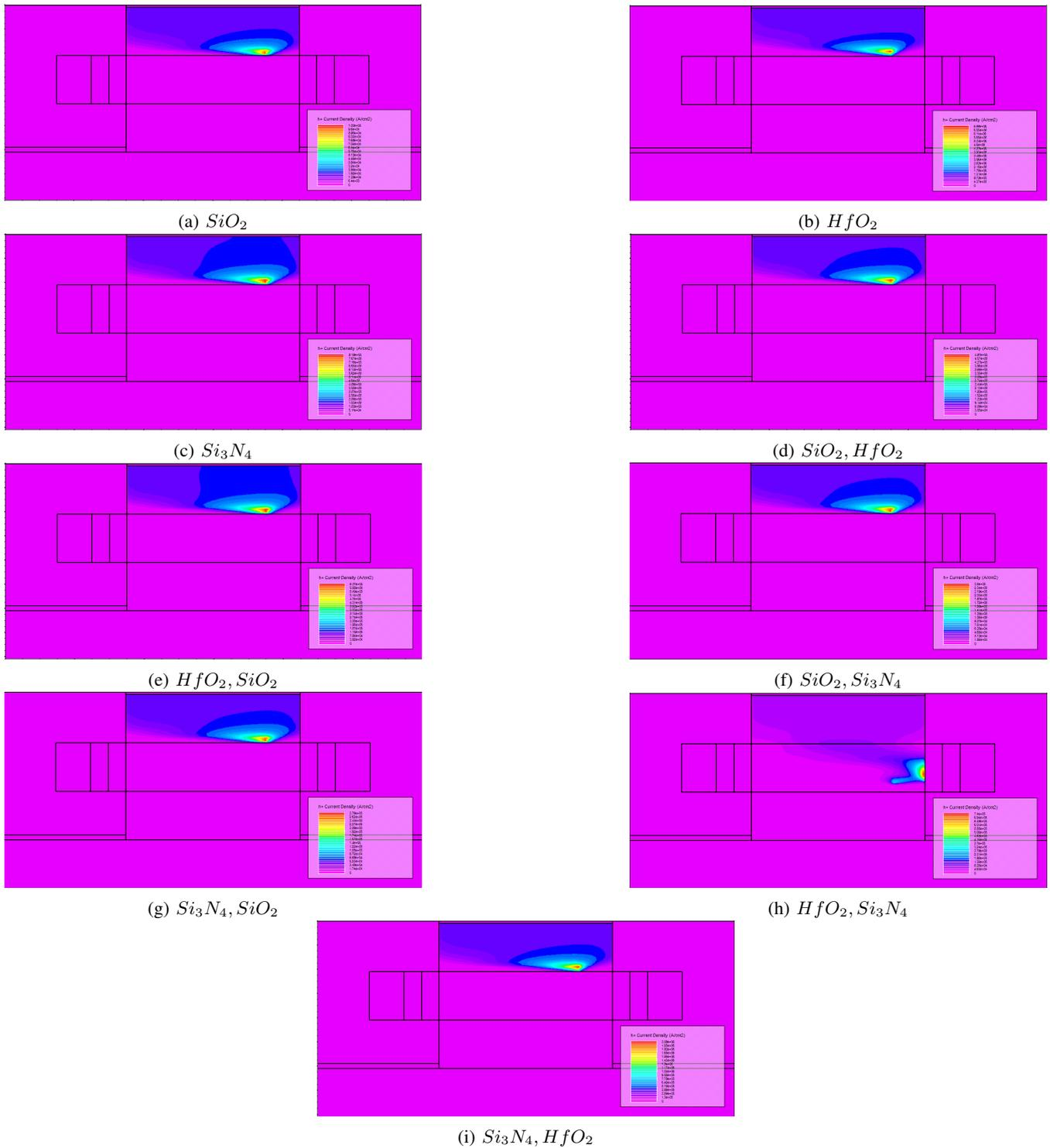
Fig. 13: Hole current density distribution for various dielectric materials, showing the effectiveness of high-k dielectrics in enhancing hole carrier mobility
