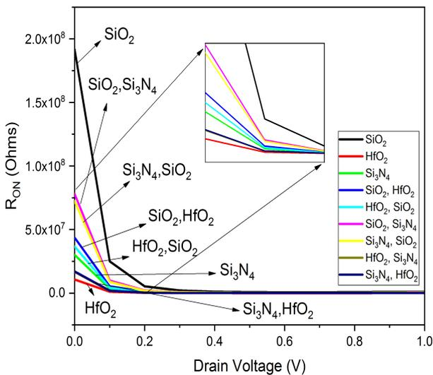
Fig. 9: Variation of On Resistance with Gate voltage for different dielectric materials
