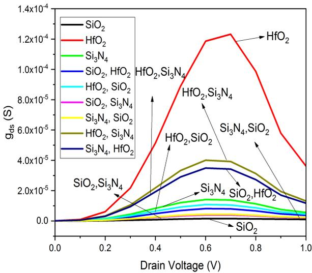
Fig. 8: Variation of Drain conductance with Gate voltage for different dielectric materials
