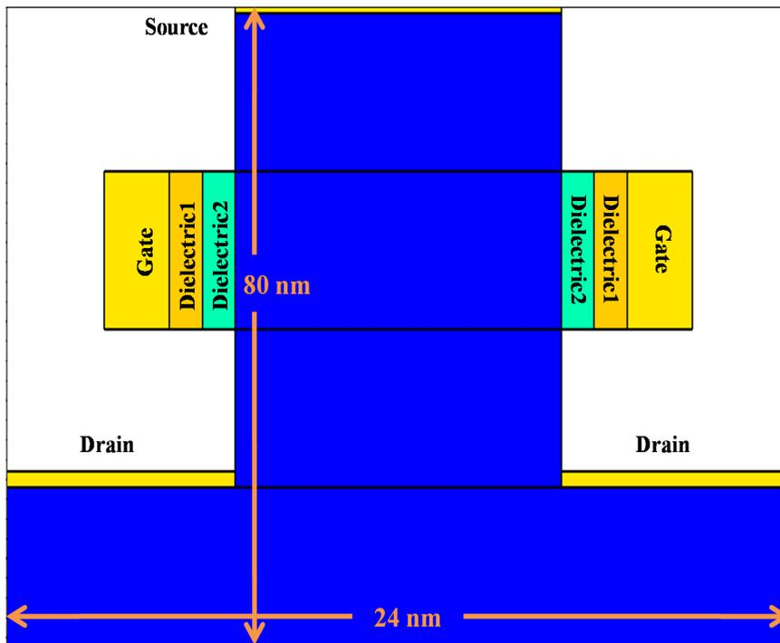
Fig. 1: Schematic representation of the proposed vertical TFET structure, highlighting the dual-gate configuration and optimized dielectric layers for enhanced tunneling efficiency
