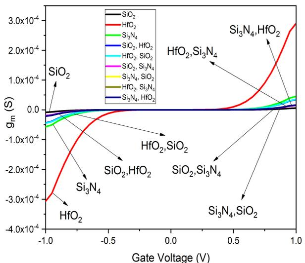
Fig. 5: Variation of Transconductance with Gate voltage for different dielectric materials
