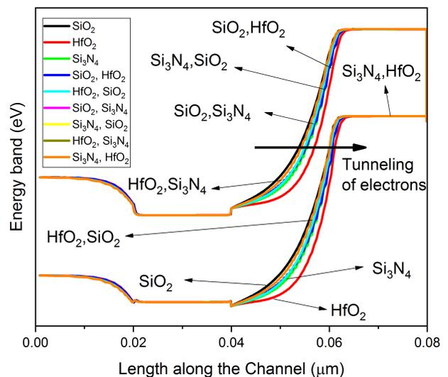
Fig. 2: Energy band diagram of the proposed TFET for different dielectric materials, illustrating variations in band alignment and tunneling barrier
