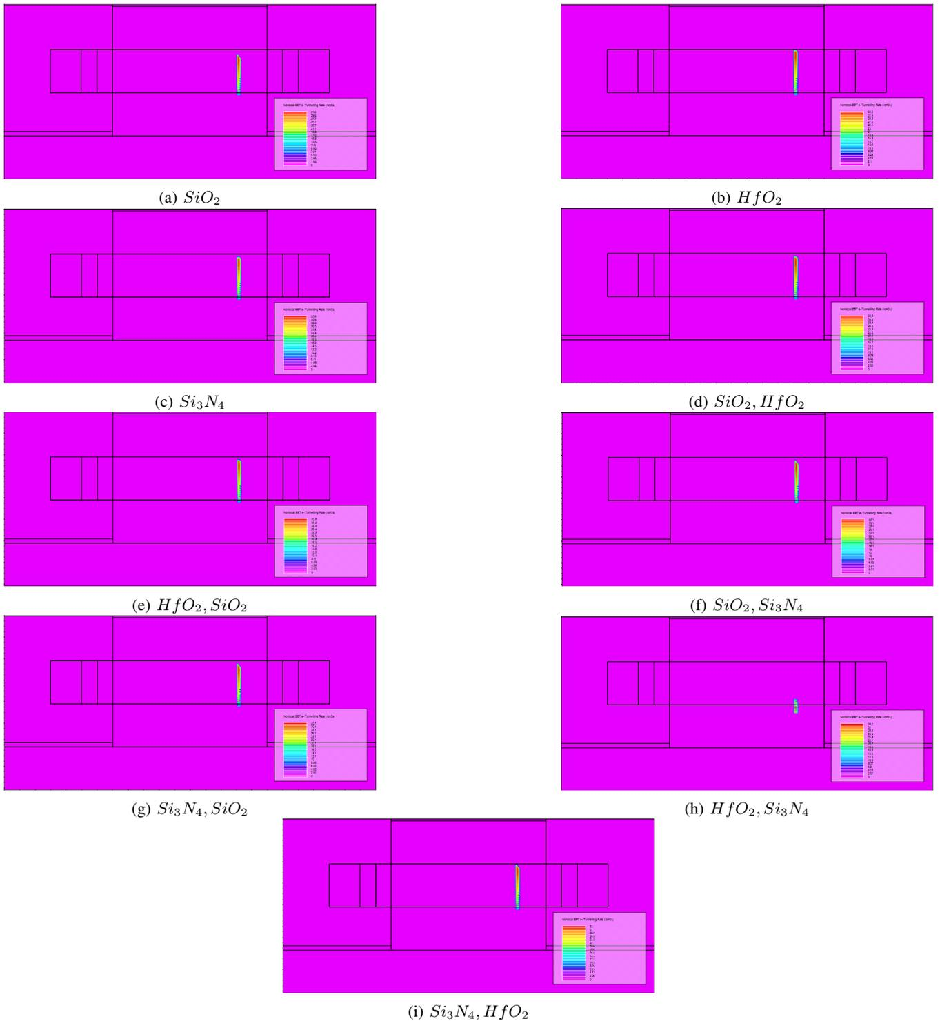
Fig. 10: Contour plots of electron band-to-band tunneling for different dielectric materials, visualizing the tunneling recombination distribution and its dependency on dielectric properties
