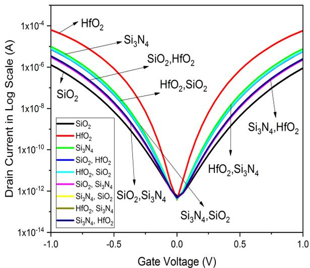
Fig. 4: Log-scale  $I_d - V_{gs}$  characteristics for different dielectric materials, emphasizing the impact of dielectrics on off-state leakage current
