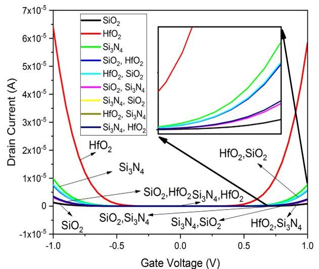
Fig. 3: Comparison of drain current characteristics for various dielectric configurations, highlighting the effect of high-k materials on gate control
