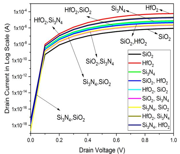
Fig. 7:  $I_d - V_{ds}$  in Log scale for different dielectric materials
