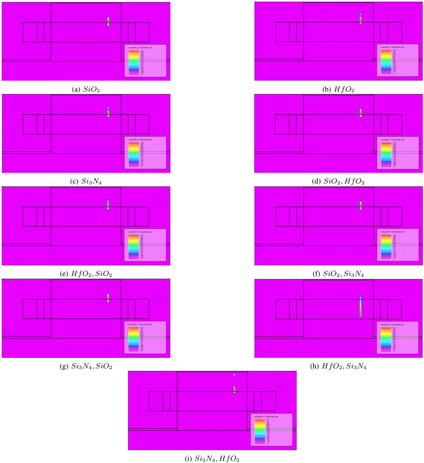
Fig. 11: Contour plots of hole band-to-band tunneling for different dielectric materials, illustrating the impact of material selection on hole transport efficiency
