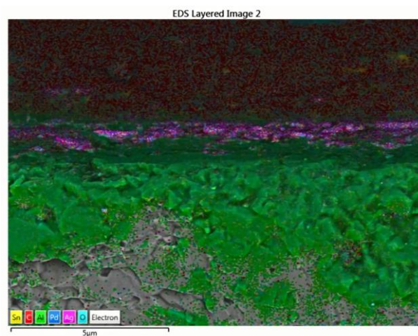
Fig. 8. Elemental distribution on the sample surface from SEM-EDS analysis (JEOL JSM IT300LV).
