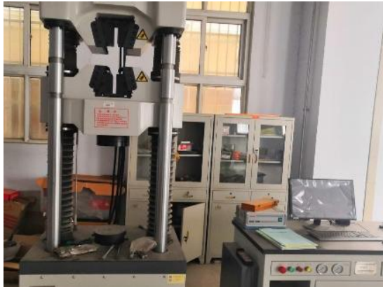
(a) Microcomputer-controlled hydraulic servo universal testing equipment
