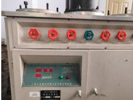
(b) Automatic pressure-regulating concrete permeability tester
