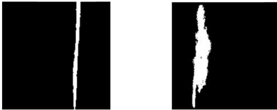
(a) Scratch enhanced segmentation (b) Inclusion enhancement segmentation Fig. 5. Segmentation results of defect enhancement images
