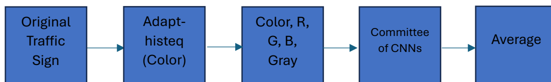
Fig. 2. The flow-chart of the proposed method: The original traffic sign image is the input. We perform color adaptive histogram equalization to the input traffic sign image, feed the enhanced image, its R, G, B channels and the grayscale image to a committee of five CNNs. We take the average of the five CNN output probabilities to determine the final class label of the input traffic sign.
